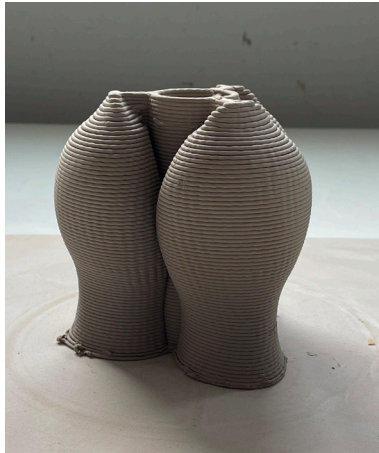
Printing vessels with curved base test 5 (elevation).
