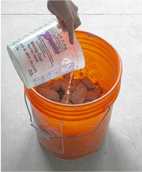
Figure 6.3.1 - 6.3.2 - Clay is stored in a bucket with excess water (left). After the clay has been left to saturate in the water, it is wedged by hand to remove air pockets (right).
