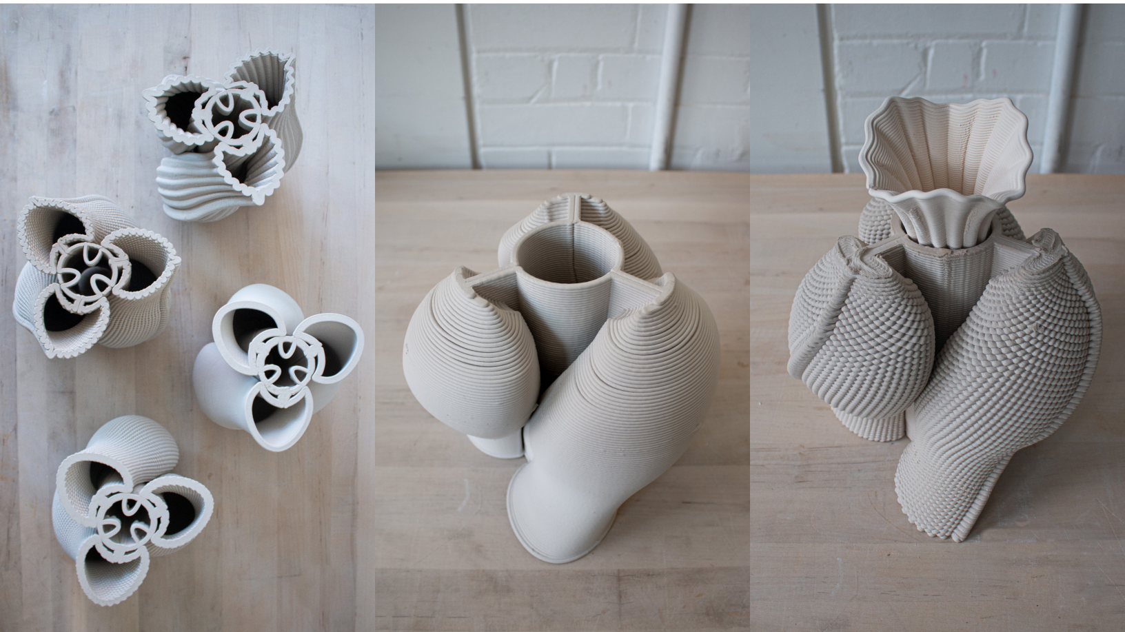
Figure 7.2.2.2.24 - 7.2.2.2.26 - Different textures and patterns were created for the plant growing components (left). A smooth tool path is prone to print layers separating during drying (middle). Disparishing the tool path to create texture minimizes print layer separation during drying (right).
