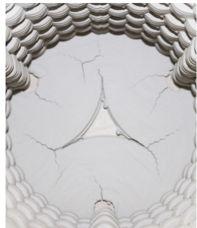
Cracking at structural base of the light shade (plan).
