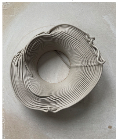
Isocurve test 7 at 1:1 experiencing collapse.
