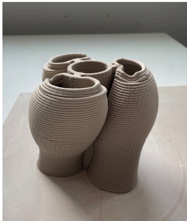
Printing vessels with curved base test 3 (elevation).
