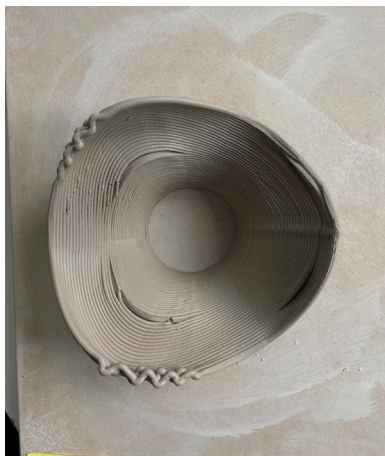
Isocurve test 7 at 1:1 experiencing distortion.
