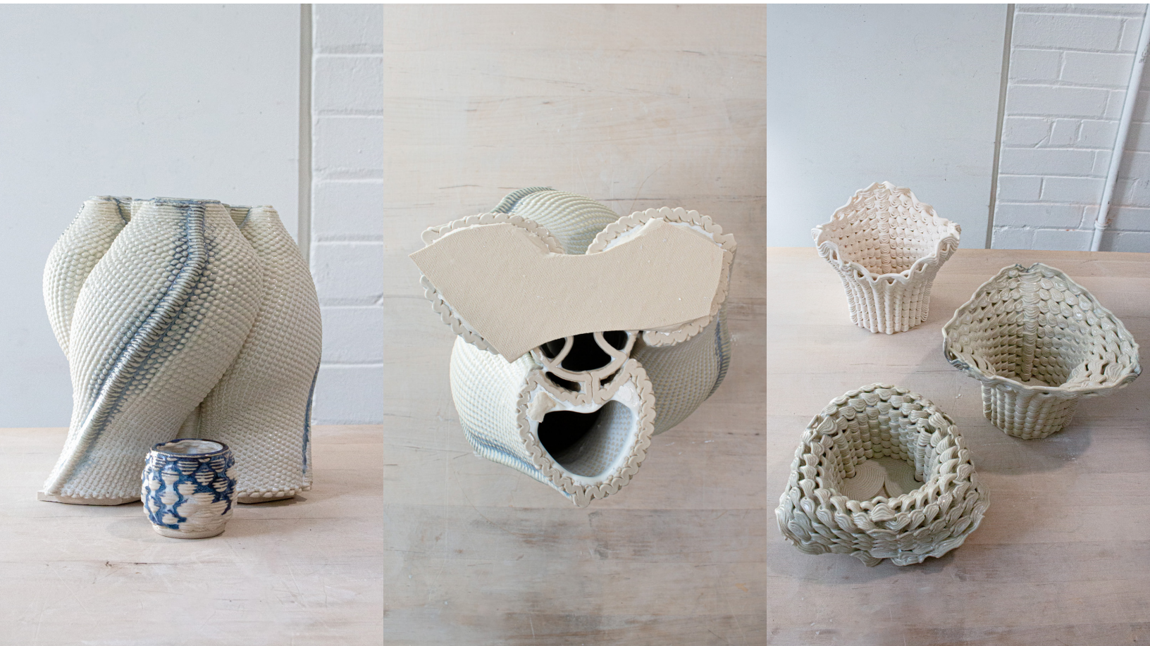
Figure 7.2.2.4.5 - 7.2.2.4.7 - The glazes on the component became patchy after firing, and produced a different result from the glaze test (left). Excess glaze in the plant vessels caused the component to fuse to the glaze tray (middle). The glaze firing caused the upper light shades to warp and collapse (right).
