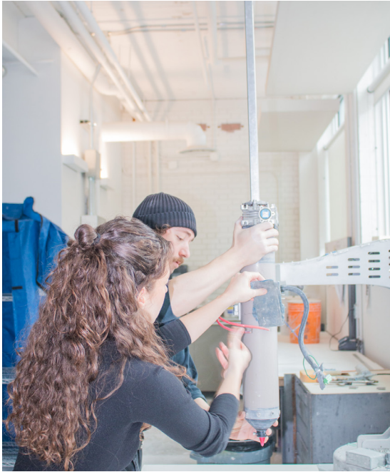
Figure 6.3.5 - 6.3.6 - The tube is then connected to the 3D printer (left). The printer is ready to print files (right).
