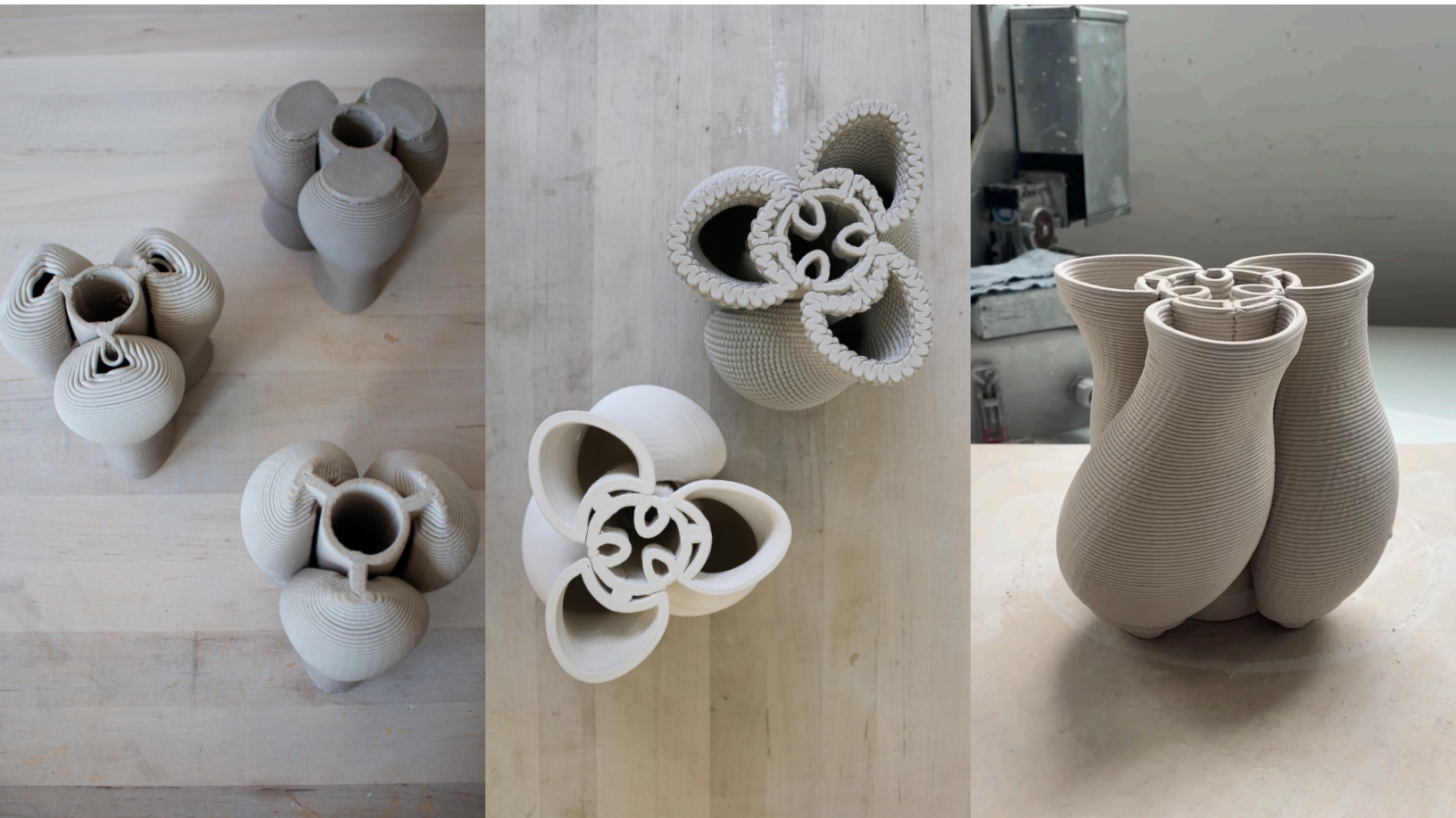
Figure 7.2.1.2.4 - 7.2.1.2.6 - Comparison between the appearance of a flat base, a delaminated base, and a laminated, curved base (left). Three structural connections are seen at the top of the vessels (middle). Front view of the plant growing component (right).
