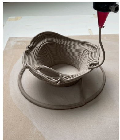
Isocurve test 8 at 1:1 experiencing collapse.
