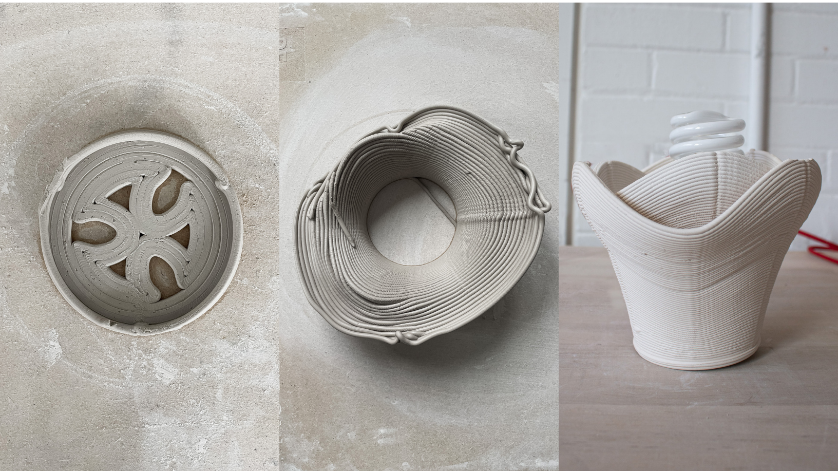
Figure 7.2.1.2.11 - 7.2.1.2.13 - The base is printed flat against the print bed with three structural openings (left). A print that experienced collapse due to changes in z-height remains intact on the right side where the structural seam is located (middle). A small shade nests inside the exterior shade and houses the light (right).
