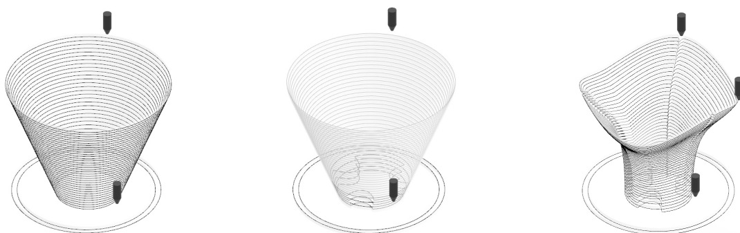
Figure 7.2.1.2.15 - 7.2.1.2.17 - A cone shape is created with a narrow base to fit within the channel of the plant growing component (left). Three structural connections are created at the base (middle). A waving curve is created at the opposite end of the cone to create the appearance of movement (right).
