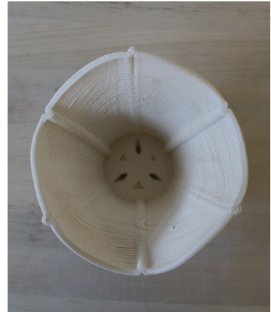
Isocurve test 9 with six ribs remains intact (plan).
