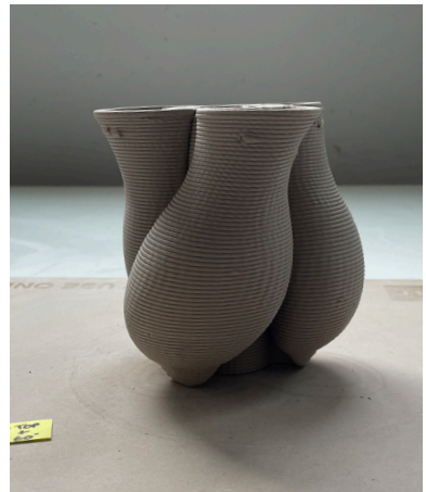
Printing vessels with curved base test 6 (elevation).
