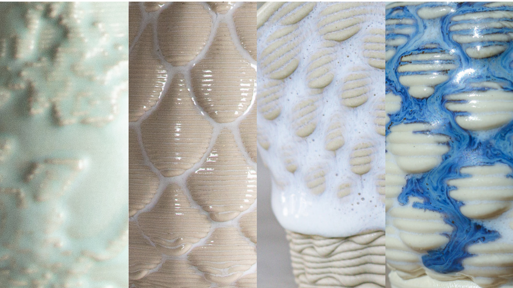
Figure 7.2.2.4.1 - 7.2.2.4.4- Matte glazes in shade wintergreen (left). Glossy glazes in shade white opal (middle left). Glaze application that was too thick (middle right). White opal and dark flux layered together (right).
