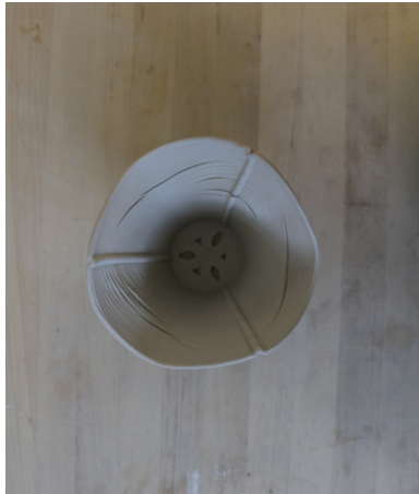
Isocurve test 8 with three ribs experiencing cracking (plan).
