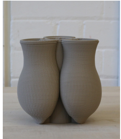
Printing vessels with curved base test 5 (elevation).
