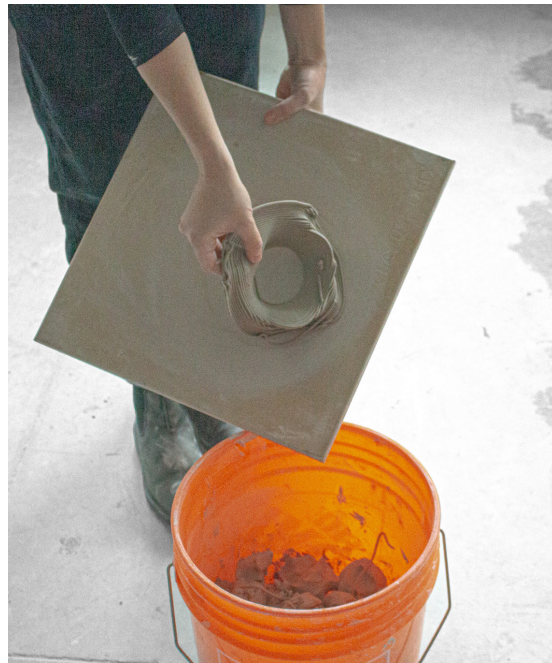
Figure 6.3.7 - 6.3.8 - A heat gun may be used to dry the clay more rapidly and allow for steep print angles to be achieved (left). Any prints that are unsuccessful are able to be reclaimed (right).
