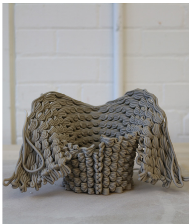
Woven texture test 3 separating at seam condition (elevation).
