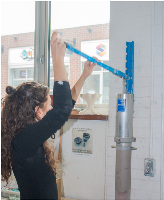
Figure 6.3.3 - 6.3.4 - The clay is shaped into cylinders and pushed through an extruder into the acrylic tube used for printing (left). The nozzle and motor are attached to the clay tube (right).
