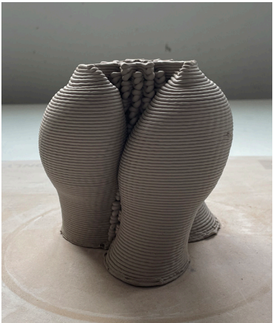
Printing vessels with curved base test 4 (elevation).
