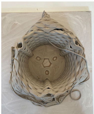
Woven texture test 4 experiencing collapse (plan).
