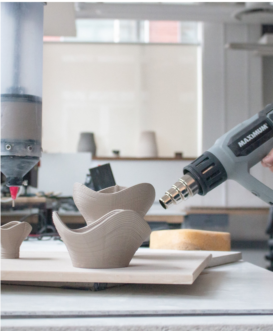
Figure 6.3.7 - 6.3.8 - A heat gun may be used to dry the clay more rapidly and allow for steep print angles to be achieved (left). Any prints that are unsuccessful are able to be reclaimed (right).
