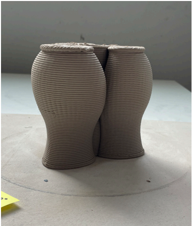
Printing vessels with flat base test 2 (elevation).
