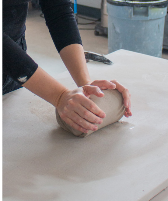
Figure 6.3.1 - 6.3.2 - Clay is stored in a bucket with excess water (left). After the clay has been left to saturate in the water, it is wedged by hand to remove air pockets (right).
