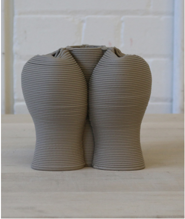
Printing vessels with curved base test 3 (elevation).
