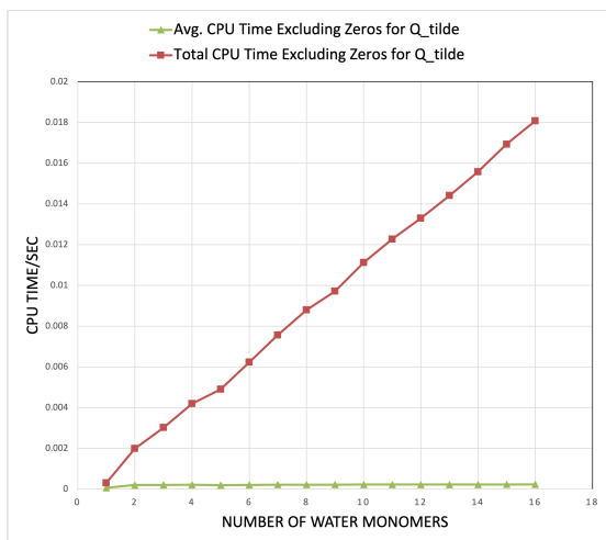
Figure 4.15: Average and Total CPU Time for Excluding Zeros in \tilde{Q}_{xy} Per LMO Slice in Polywater Systems (H_2O)_n using the cc-pVTZ Basis Set and cc-pvtz-jkfit Auxiliary Basis Set ( \alpha = 1.0 ).
