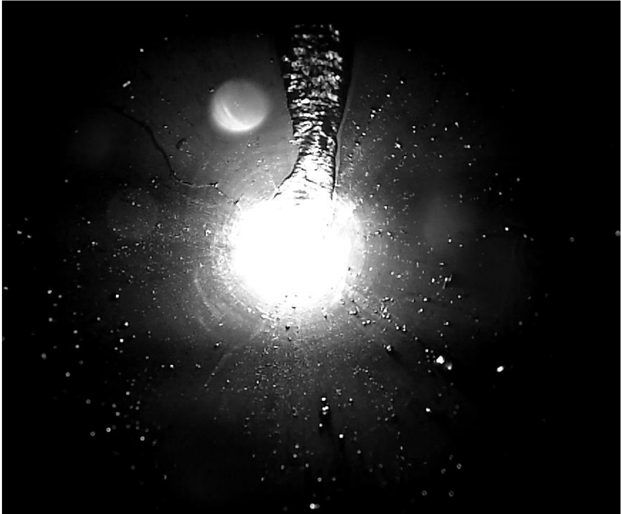
Figure 3-5 Stable partial wetting of the drain pipe observed inside a 7.6cm diameter DWHR system at a flow rate of 2 LPM.
