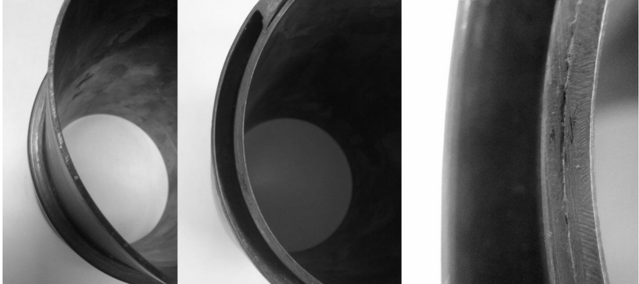
Figure 4-1 Typical construction of a 10.2 cm DWHR system, where the leftmost picture shows the coils wrapped around the drain pipe, the picture in the middle shows a coil that was cut and the rightmost picture shows the contact interface between the coil and the drain pipe.
