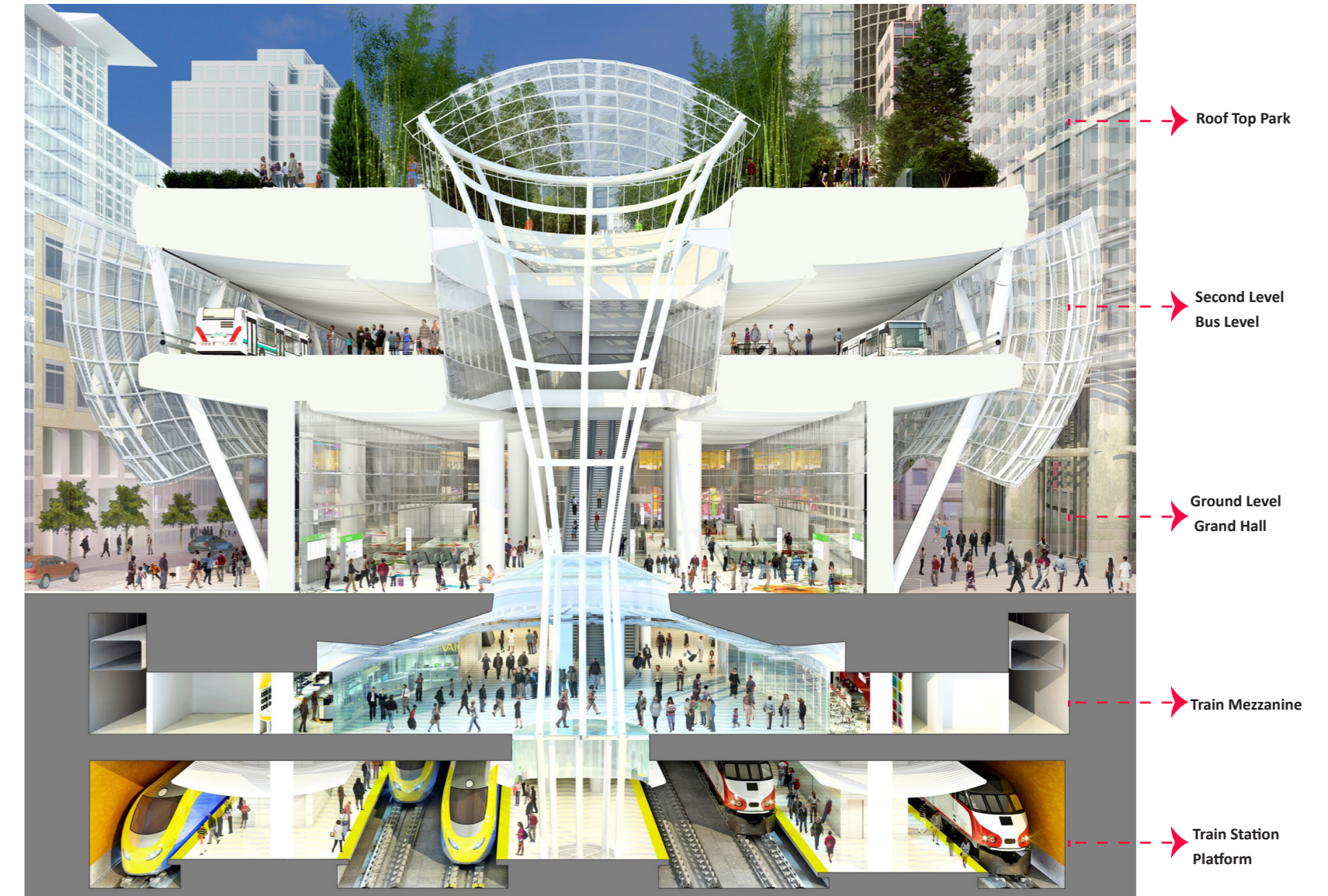
3.13 Cross Section View of the new Transbay Transit Centre ~ The Multi Modal Transit Hub has five levels and connects eleven transit systems with different functions for passengers.
