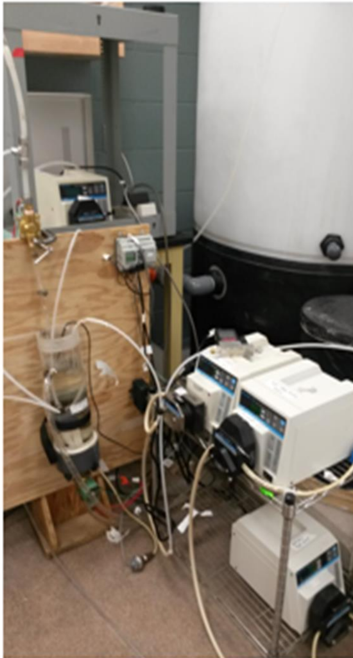
Figure A. 5 Ultrafiltration module and permeation pump
