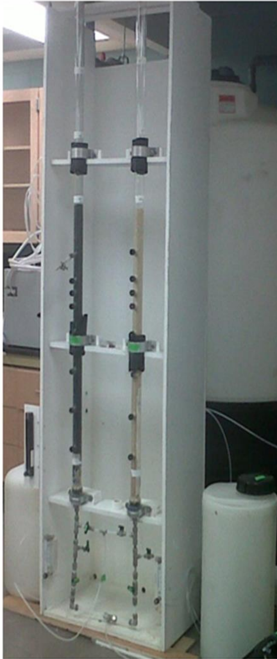
Figure A. 2 Main biofiltration experimental set-up
