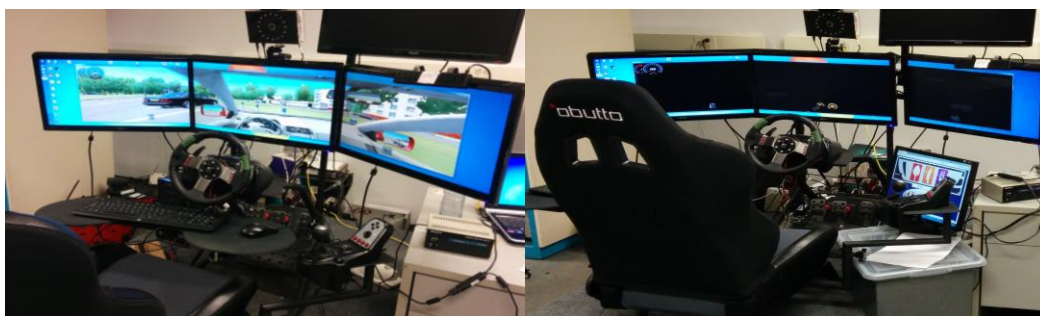
Figure 4.16: The driving simulator with Scenarios 1 & 2
