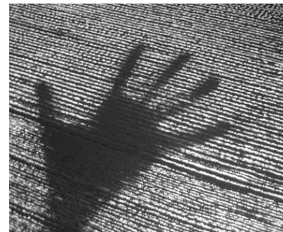
Figure 4.25 “Translucent Concrete Wall”. By Andreas Bittis. 2007. Unspecified Location.
