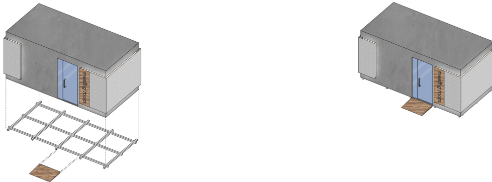
Figure 4.63 - "Pods on the Ground". Unlike pods lifted into the lattice space, pods on the ground level do not need the added structure. However an individual 'micro lattice' is place beneath the pods for enhanced separation.
