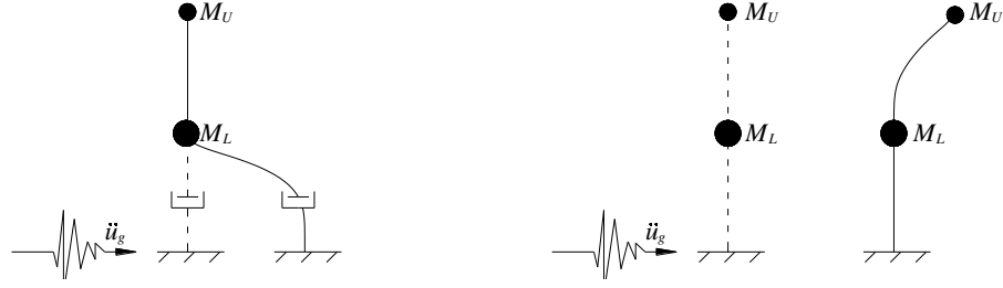
(a) extremely flexible lower structure ( R_k \rightarrow 0 ) (b) extremely stiff lower structure ( R_k \geq R_{kU2stg} )
