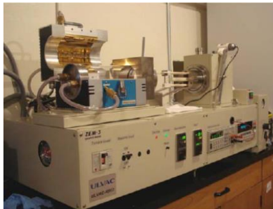
Figure 2.11 ZEM-3 (ULVAC-RIKO) electrical resistivity and Seebeck coefficient measurements instrument.
