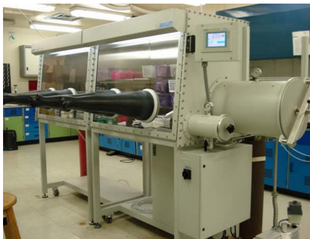
Figure 2.4 Ar atmosphere glove box with oxygen and moisture level of less than 2 ppm.
