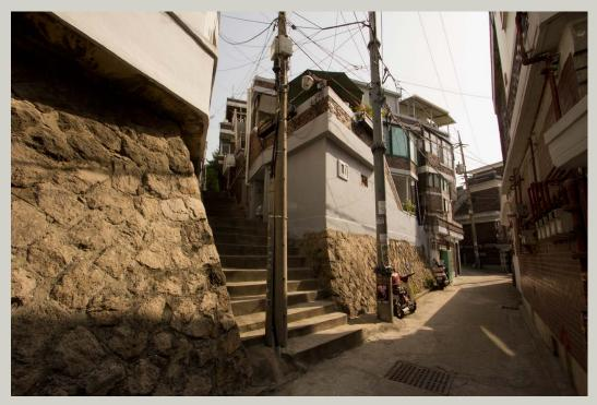
Figure 3.140 An area where double-storey houses are built on drastically steep slopes. Consequently, elevated bases are built higher in order to overcome the height difference, making the buildings float above one's head.
