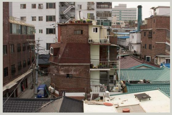
*Figure 3.59* Different and less sturdy material suggests a horizontal extension. Railed balconies wrap around, connected by stairs built with similar materials.
