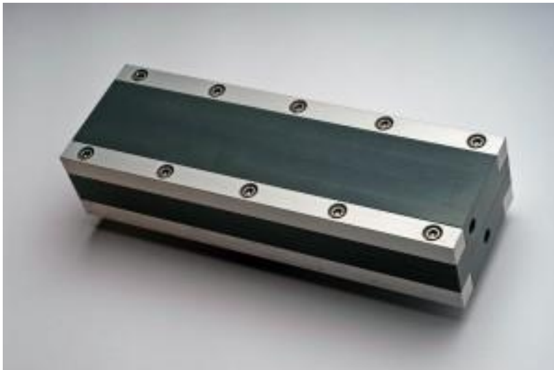
Figure 2-4 A photo of the membrane fouling simulator (MFS) units used for biofouling detection
