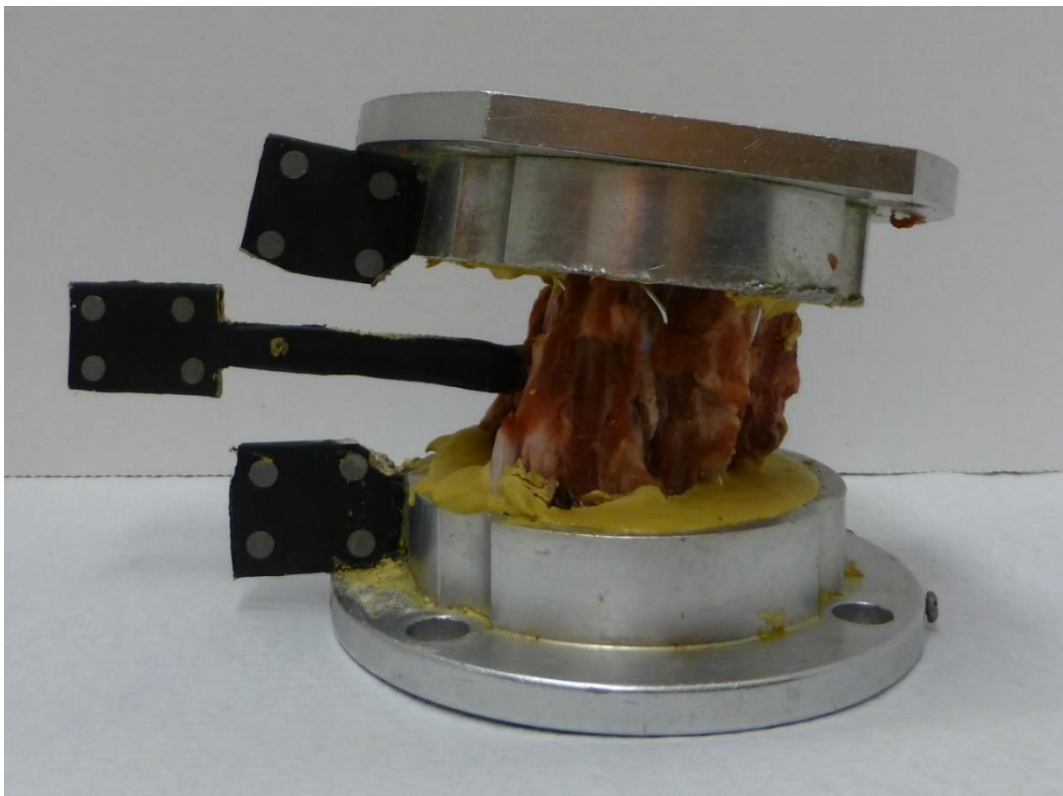
Figure 4.2 Rigid body marker setup on spine specimens. Two rigid bodies were fixed to the superior and inferior mounting cups (these did not move relative to the superior and inferior vertebral bodies) while another rigid body was fixed via small wood screws to the middle vertebral body.
