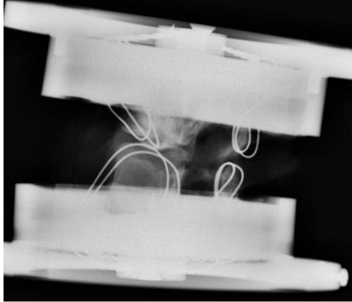
Figure 5.8 Specimen post-fracture, the dye can be seen in the superior vertebral body indicating a superior endplate fracture.
