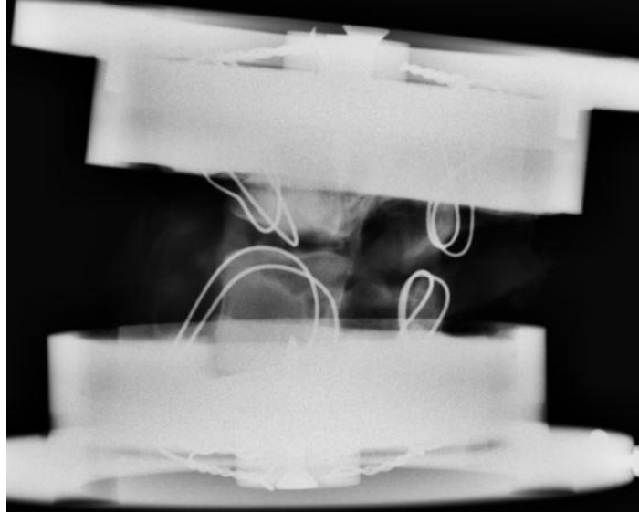
Figure 5.10 Specimen post-hydrogel injection, increased disc height as a result of injection can be seen.
