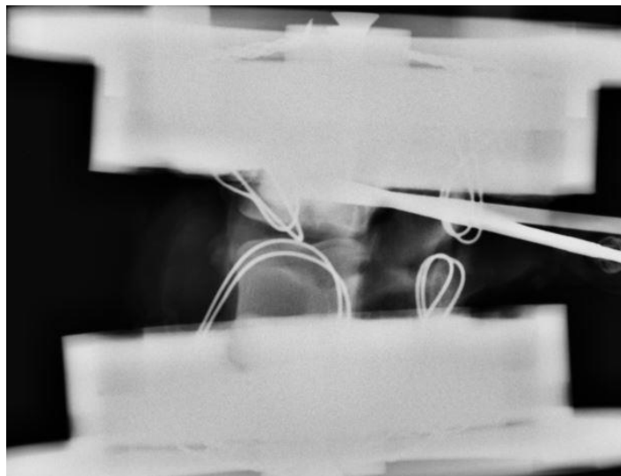
Figure 5.11 Specimen post PMMA injection. The cement was radio-opaque and its injection site can be visualized.
