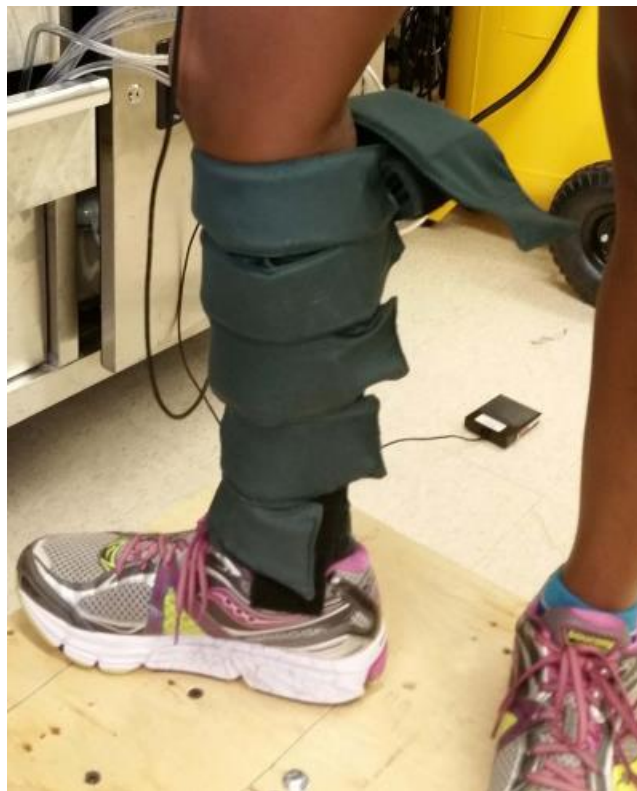
Figure 11: Five out of six pneumatic cuffs wrapped around the calf portion of the leg
