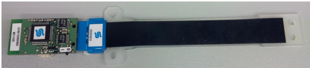
Figure 22: StretchSense standard stretch-mode sensor and circuit board
