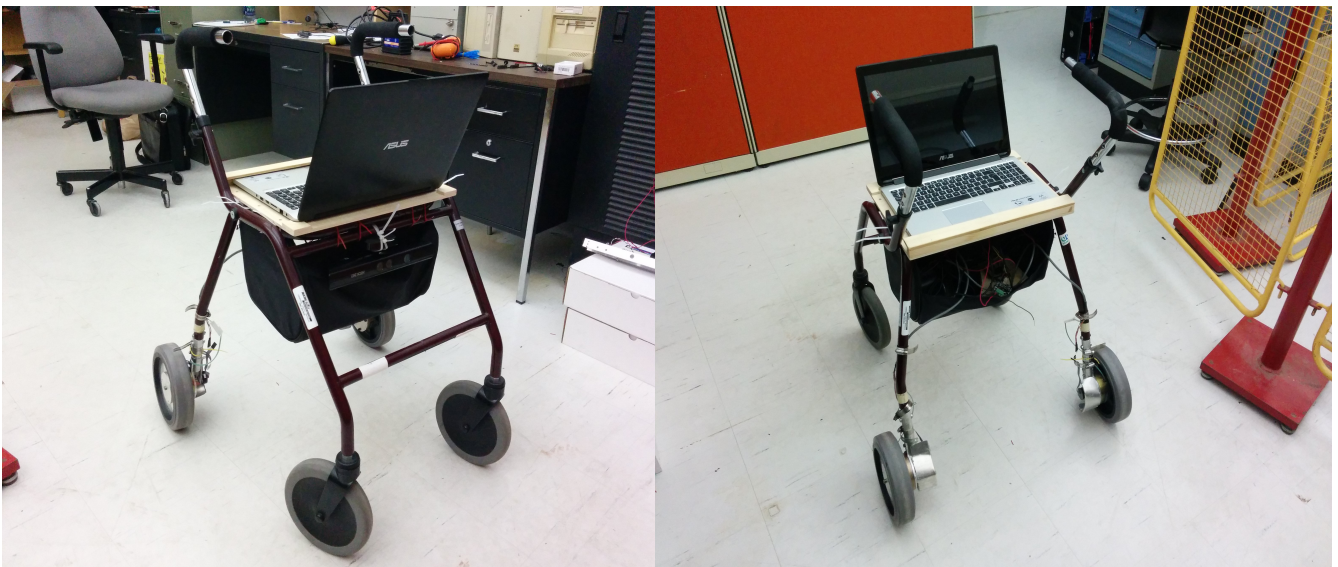
Figure 3.1: Front and back views of the novel intelligent assisted-walking device.
