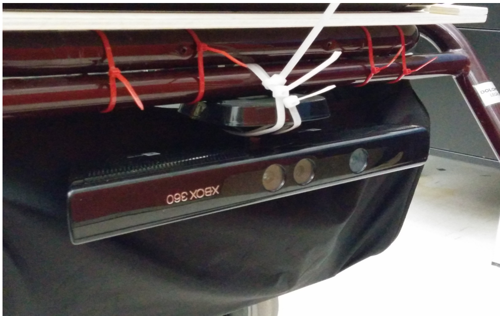
Figure 3.7: The Microsoft Kinect mounted on the front of the walker.
