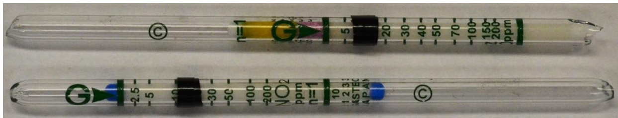
Figure 4-34: NO and NO 2 concentrations measured using Gastec STR-800 tubes during suppression of wood crib fire using a StatX aerosol (650 Seconds)
