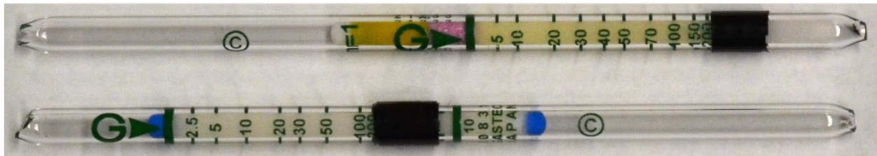
Figure 4-26: NO and NO 2 concentrations measured using Gastec STR-800 tubes during suppression of a diesel fire using a DSPA aerosol (500 seconds)
