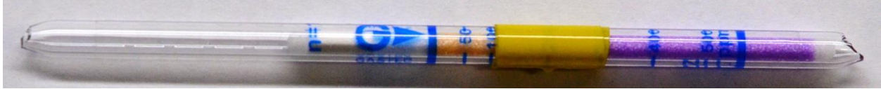
Figure 4-10: NH 3 concentration measured using a Gastec STR-800 tube during suppression of a diesel fire using a StatX aerosol unit inside the UW burn room (640 seconds)
