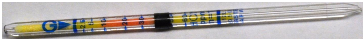
Figure 4-59: Measured HCN concentrations for cold agent discharge (DSPA-Test F, 400 seconds)
