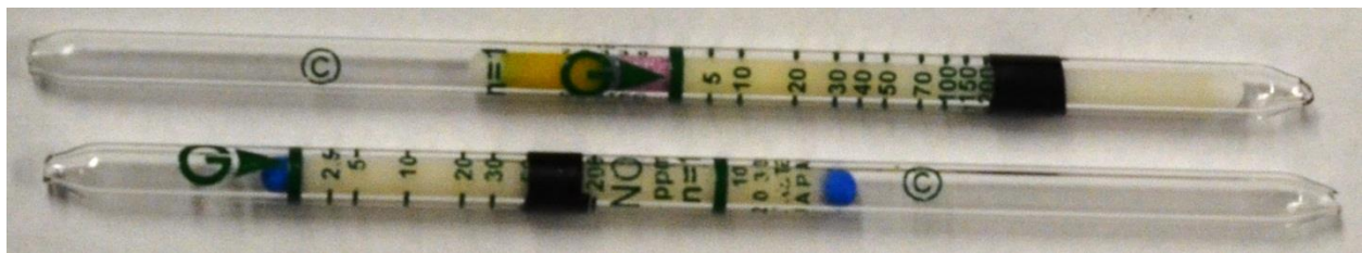
Figure 4-54: Measured NO x concentrations for cold agent discharge (DSPA-Test E, 210 seconds)
