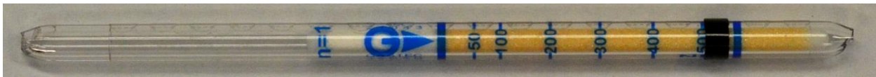
Figure 4-39: NH 3 concentration measured using a Gastec STR-800 tube during suppression of a Softwood using a DSPA aerosol unit (960 seconds)
