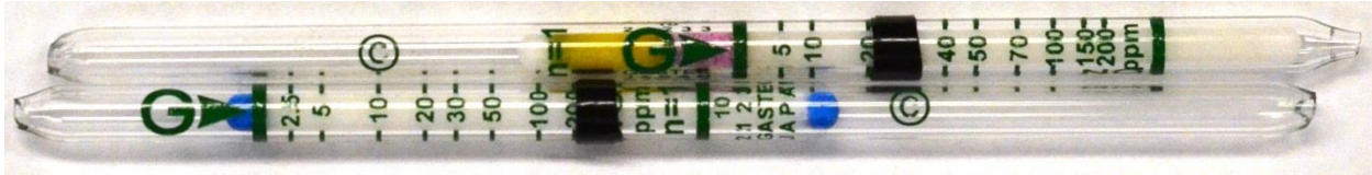
Figure 4-38: NO and NO 2 concentrations measured using Gastec STR-800 tubes during suppression of wood crib burn using a DSPA aerosol unit (710 seconds)
