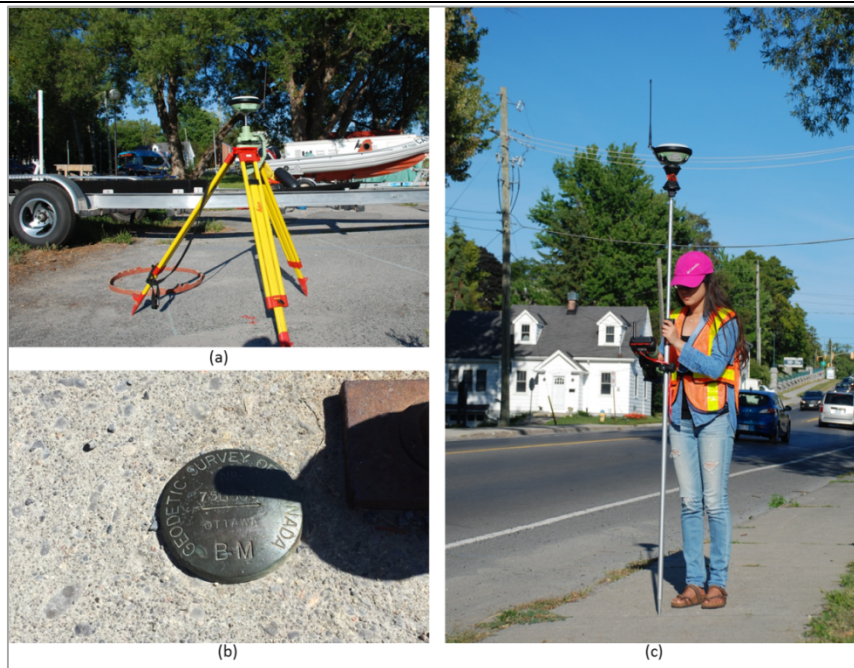
Figure 3.6: Field surveys. (a) is the GPS used as the base station, (b) is the benchmark 75U501, and (c) is the GPS used as the rover in the survey.
