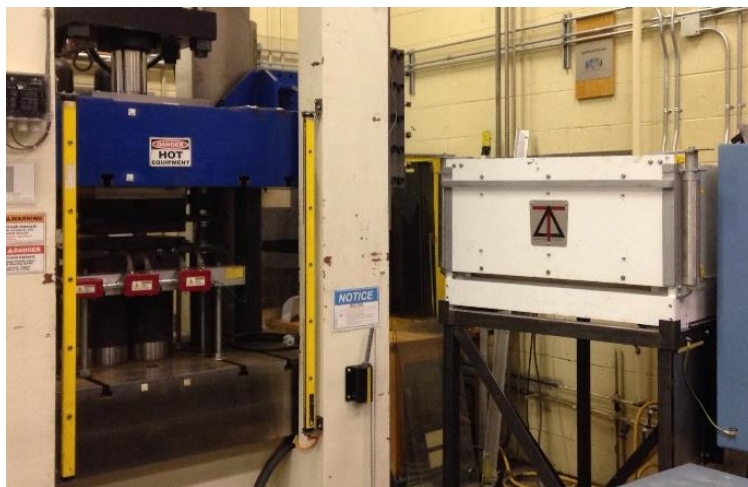
Figure 3-1: UofWaterloo Hydraulics Lab - Mini Macrodyne Press and Front Loading Furnace
