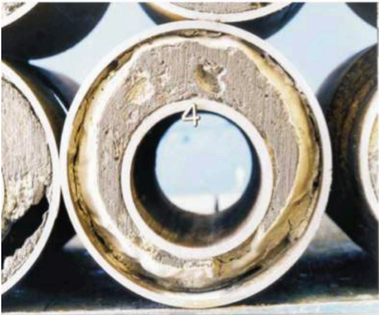
Figure 2.9. Microannulus resulting from poor drilling fluid displacement. An eccentric casing significantly exacerbated the problem (Watson, 2004)
