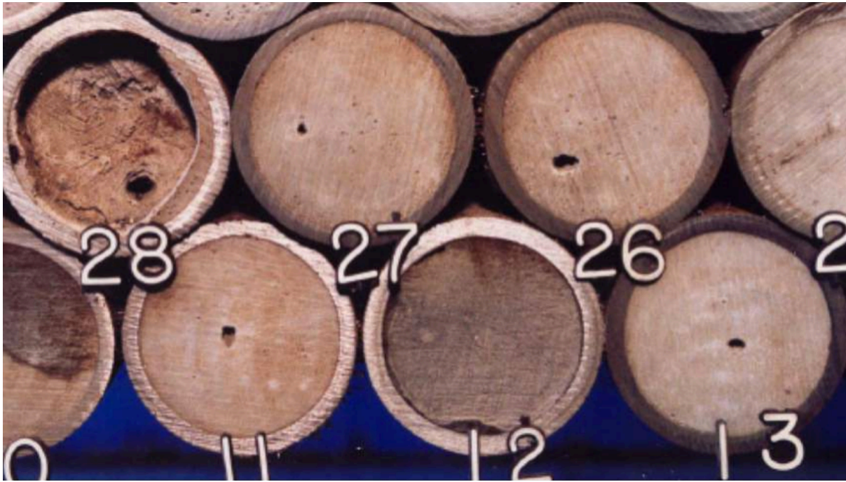
Figure 2.10. Channels formed in cement sheath as a result of fluid invasion during cement set (Watson, 2004)
