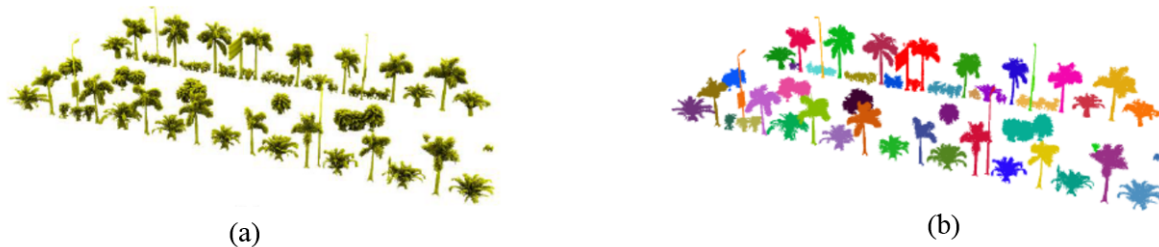
Figure 3-7 Demo of conditional Euclidean clustering algorithm (Yu et al., 2015)
