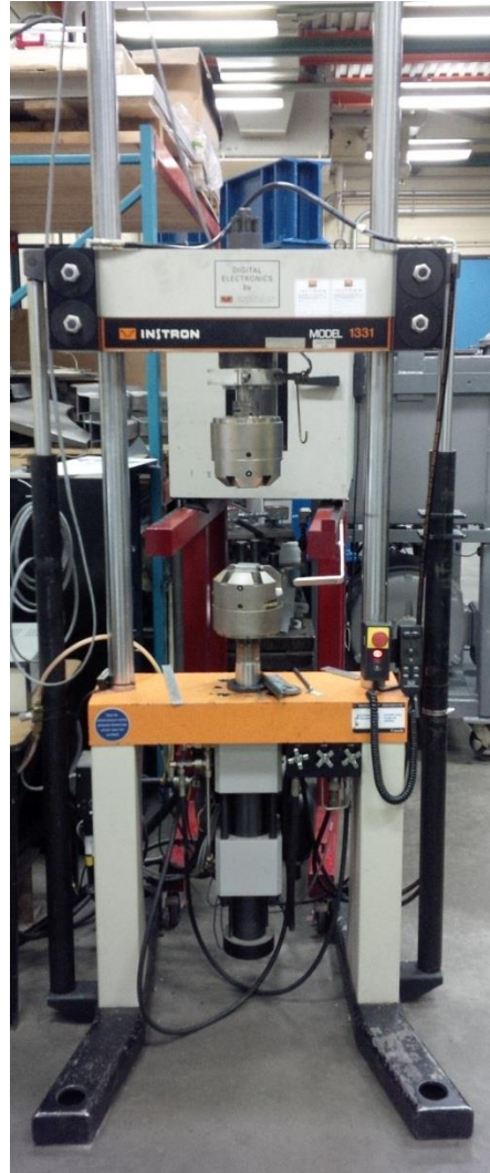
Figure 18: Instron Model 1331 servohydraulic mechanical testing apparatus
