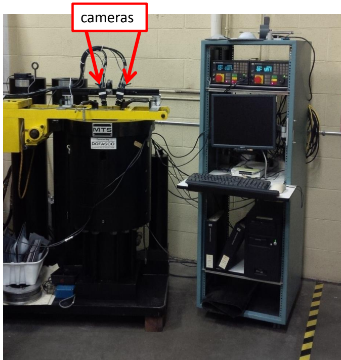
Figure 21: MTS dome tester apparatus
