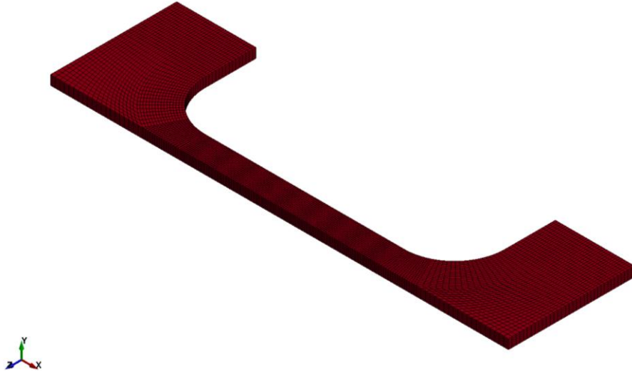
Figure 31: Mesh for quarter-symmetry uniaxial tensile model
