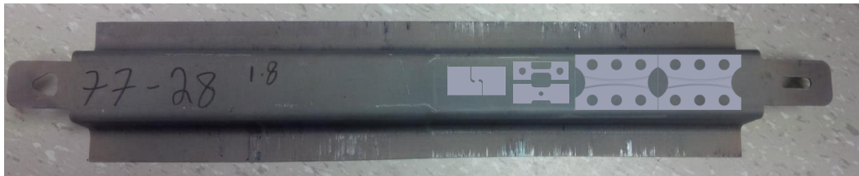
Figure 13: Depiction of specimens produced from tailored hot stamped parts formed at 400 and 700 °C. Specimens shown, from left to right: mini shear, mini dog bone and hole tensile, and two butterfly specimens
