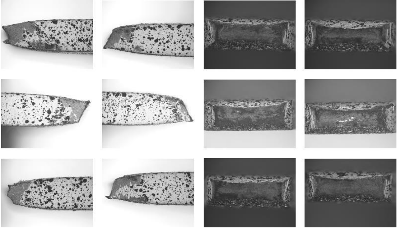
4a notch – fully bainitic
