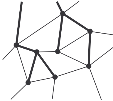
Figure 5.6: Illustration of steepest edges, assuming \zeta faces the top of the page.
