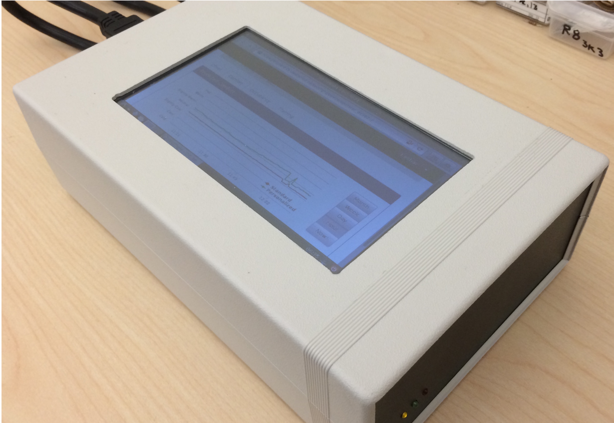
Figure 4.4: For isolated installations of OpenTherm, a 7-inch touch screen LCD is mounted on the actuation box. This LCD is connected to the RPi inside the box and provides a local GUI to the user. In this configuration, which has the best privacy protection, occupancy data remains physically in the office.
