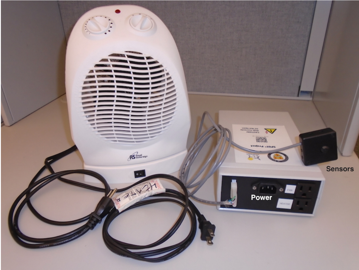
Figure 4.1: Hardware components of actuation and sensing in OpenTherm. The fan/heater is shown on the left side, and the actuation box is on the right side. In this picture, the two independent power cords of the modified fan/heater are connected to the box. The modular design of the box allows usage of different types of fans and heaters.
