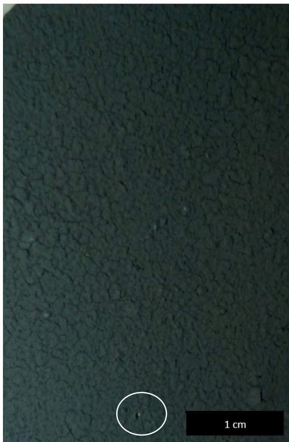
Figure 10: Digital photograph of attempted 4\text{mg cm}^{-2} loading small particle NPC electrode with 15% binder, pinhole indicated with white circle
