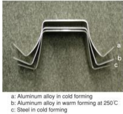
Figure 9: Cold and warm hat-shaped parts of 5xxx series aluminum alloy and cold formed mild steel alloy [21].
