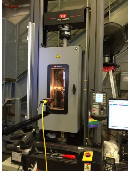
Figure 11: Experimental set-up for the tensile tests.
