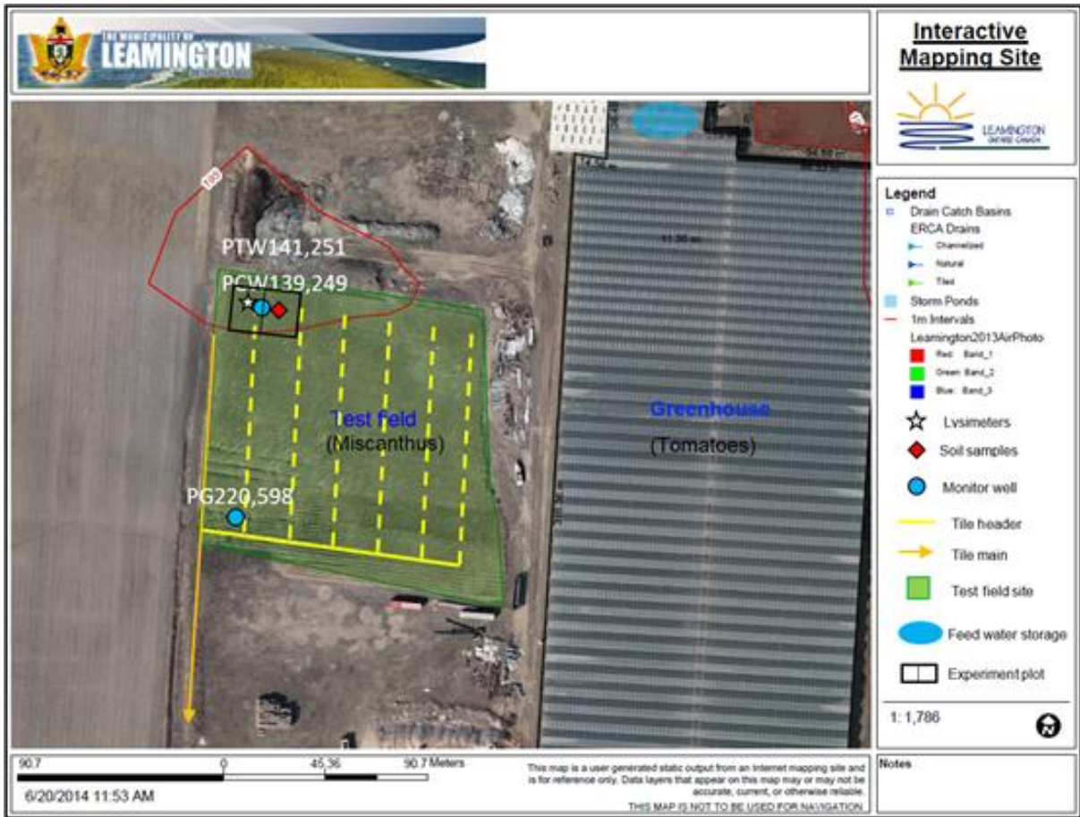
Figure A.1 Detailed site plan of the Prism Farms site showing the location of the greenhouse, the potential nutrient feed water land application site, infiltration test plot sites and relevant instrumentation and field characteristics
