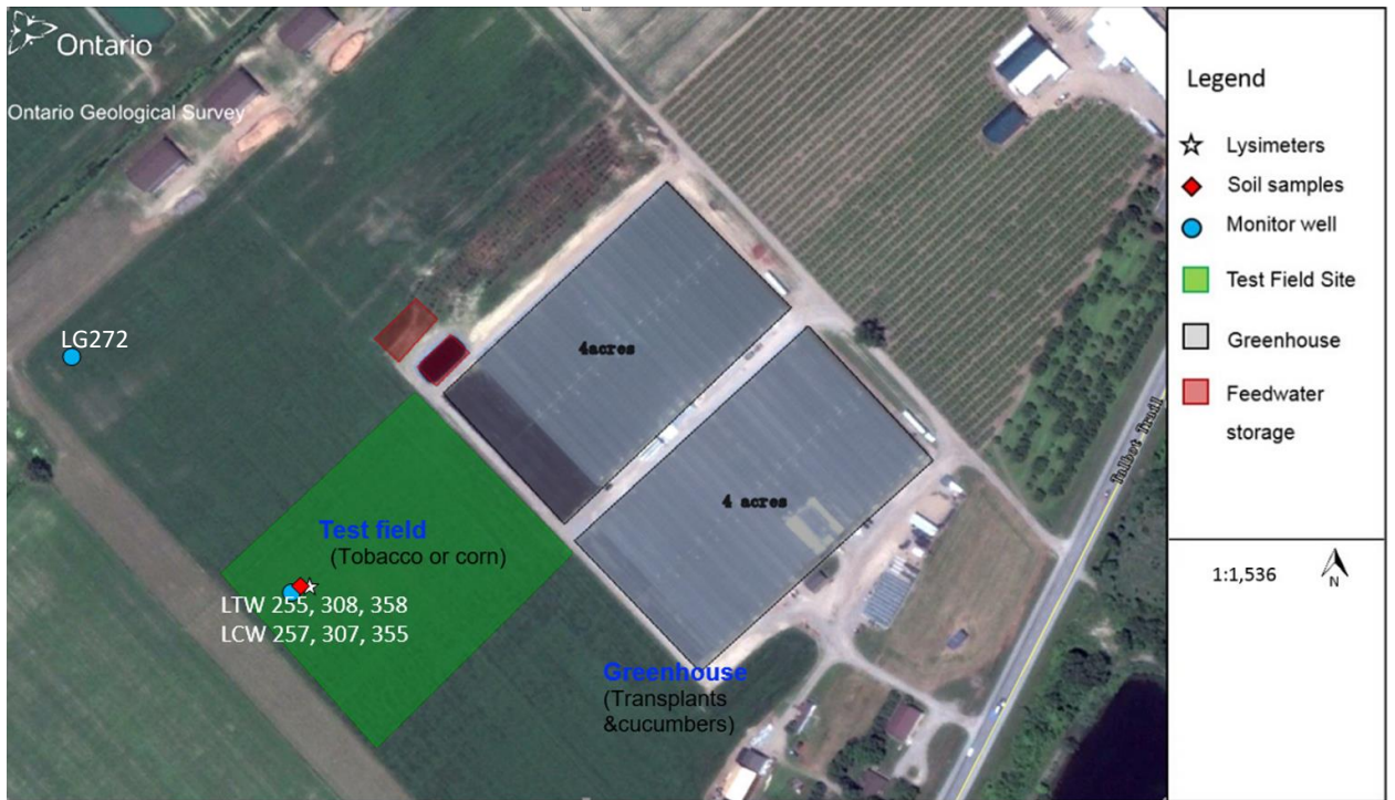
Figure A. 8 Detailed site plan of the Lakeview Greenhouse and Farm site showing the location of the greenhouse, the potential nutrient feedwater land application site, infiltration test plot sites and relevant instrumentation and field characteristics.
