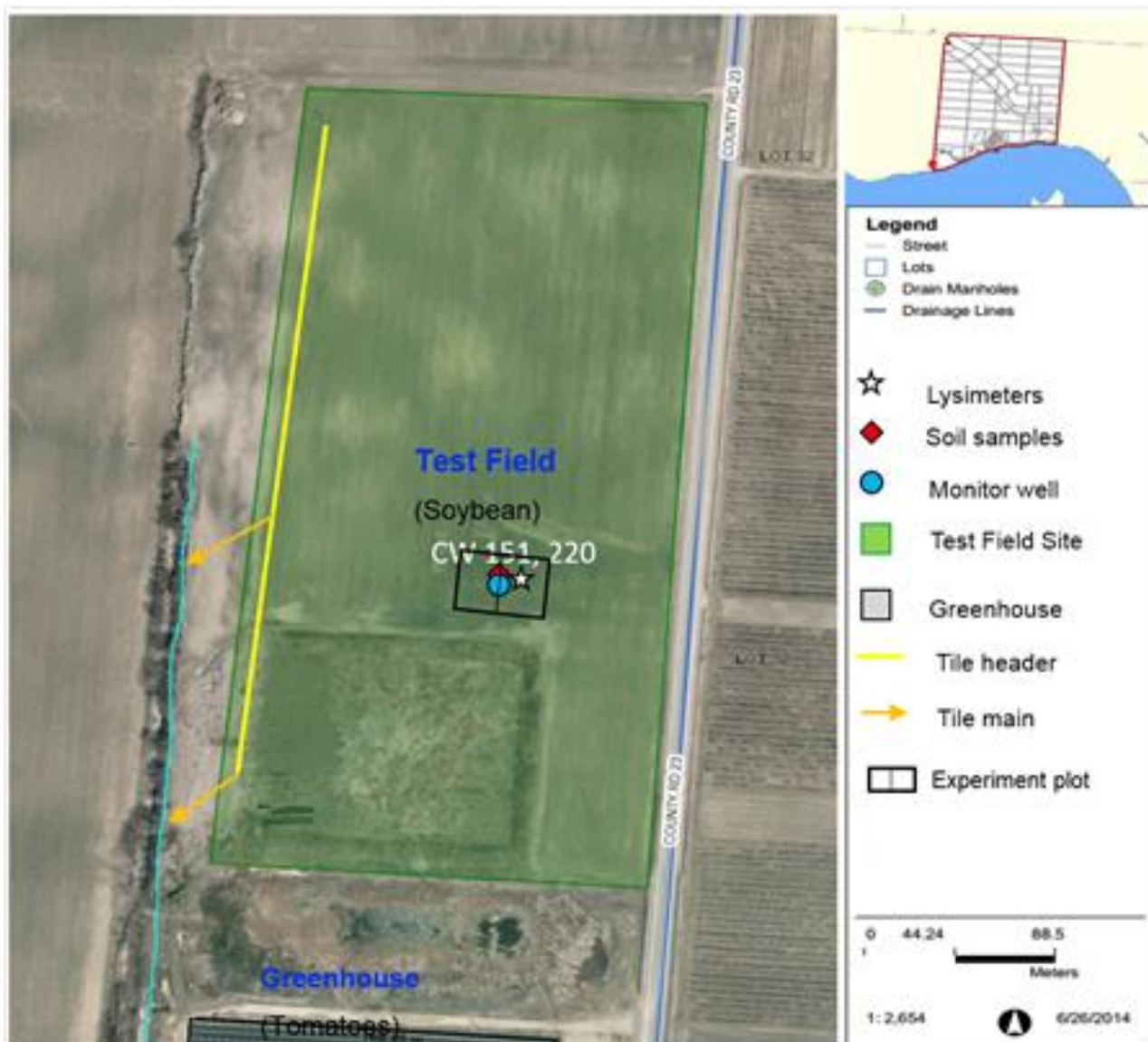
Figure A.4 Detailed site plan of the Cecelia Acres site showing the location of the greenhouse, the potential nutrient feedwater land application site, infiltration test plot sites and relevant instrumentation and field characteristics
