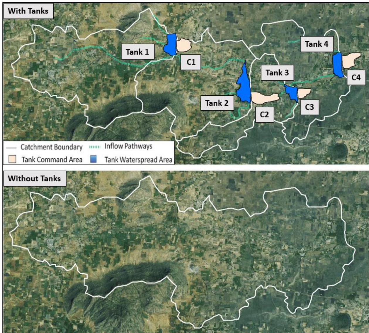
Figure 3.9: Catchment water balance scenarios for (a) the with-tank (WT) scenario to represent current conditions within the catchment (i.e., four existing tanks); and (b) the no-tank (NT) scenario, with all other conditions (e.g., rainfall, ET on the catchment area) being the same.
