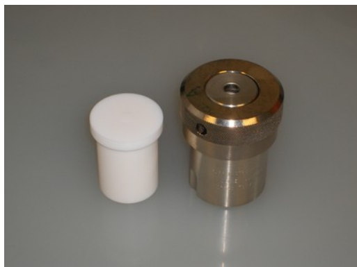
Figure 2.3: Teflon-lined autoclave used to synthesize NiSb nanoparticles and to coat them on bulk \text{Ni}_{0.05}\text{Mo}_3\text{Sb}_{5.4}\text{Te}_{1.6} .
