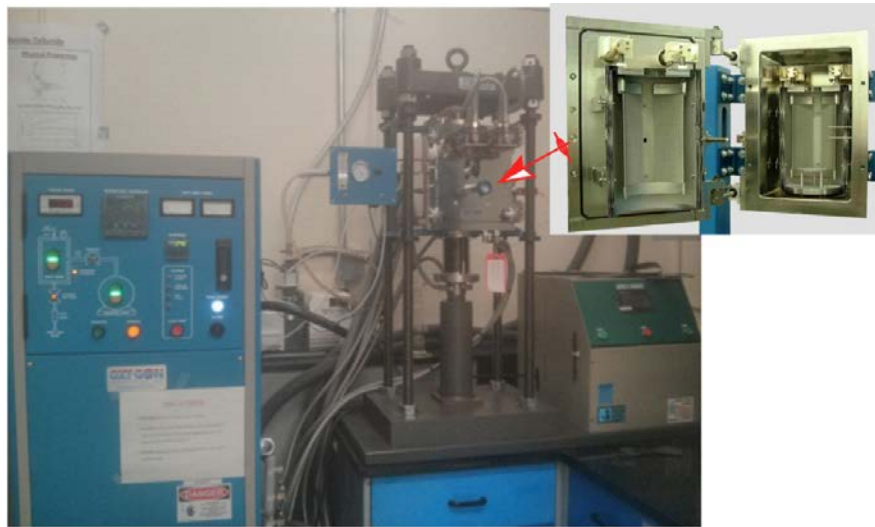
Figure 2.15: Uniaxial hot-pressing machine. Inset shows heat zone.
