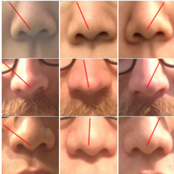
Figure 5.4: Lighting direction analysis algorithm test using photos of real people: red lines are the estimated lighting direction; left column: the light comes from top-left; middle column: the light comes from top-middle; right column: the light comes from top-right.
