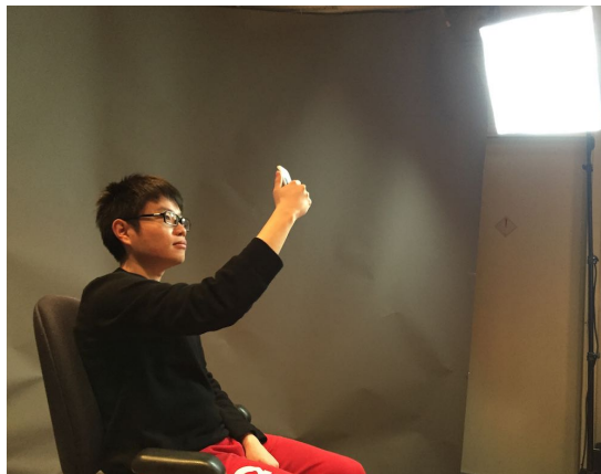
(b) The participant sits in the chair, moves the camera to manipulate face size , face position or rotates to adjust lighting direction .
