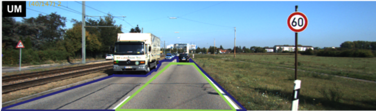
Figure 1.1: Lane Detection Focus on Drivability: Example ground truth from the [11]. The focus here is on detecting only the immediately drivable portions of the roadway (blue) and the ego-lane (green).
