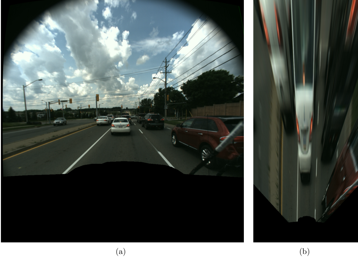
Figure 3.1: BEV Distortions: (a) An image of a road scene containing obstacles and out-of-plane features. (b) The resulting Bird's Eye View image. Even relatively small features in the source image produce large streaks if they occur far enough above the ground plane. The rear window of the leading vehicle is not prominent in the source image but takes up roughly a third of the BEV image.
