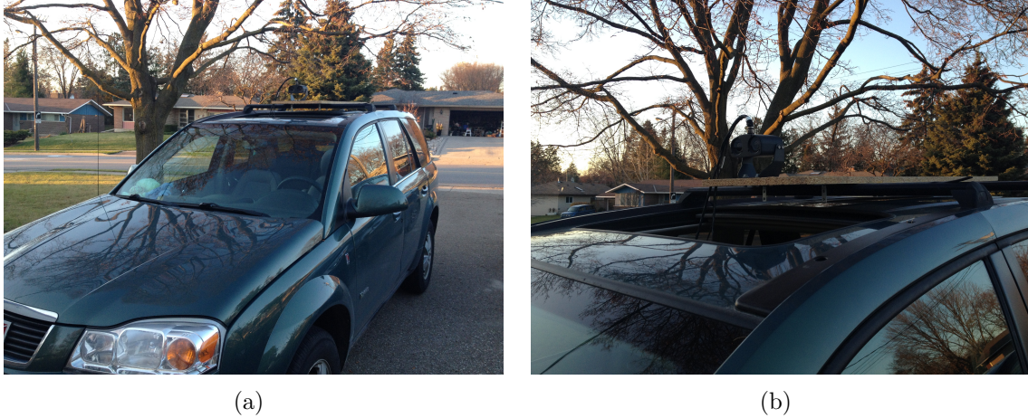
Figure 4.4: Data Capture Configuration for WARR Dataset: (a) The platform used for capturing the dataset. (b) A closer view of the camera.
