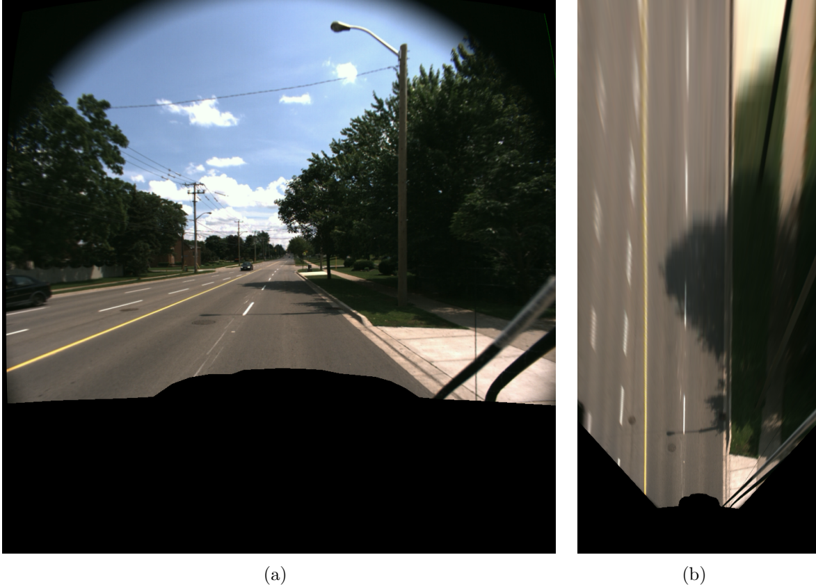
Figure 2.1: Example of the Bird's Eye View: (a) A monocular image of a road scene. (b) The corresponding Bird's Eye View image obtained using the known intrinsic calibration parameters of the camera and estimated extrinsic parameters relative to the ground plane.
