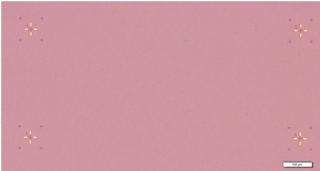
Figure 19: Optical images of alignment markers. Large crosses are alignment makers, while small ones alignment markers for write field alignment.
