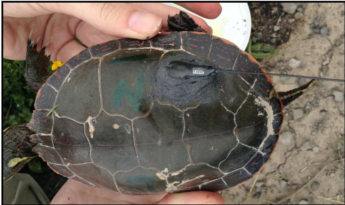
Figure 4.3 : A painted turtle with a 3.6 g glue-on radio transmitter attached to the carapace. As seen in this photo, the transmitter is attached to a lower right costal carapacial scute, and smoothed over with a waterproof epoxy to prevent snagging (photo: B. Brown).
