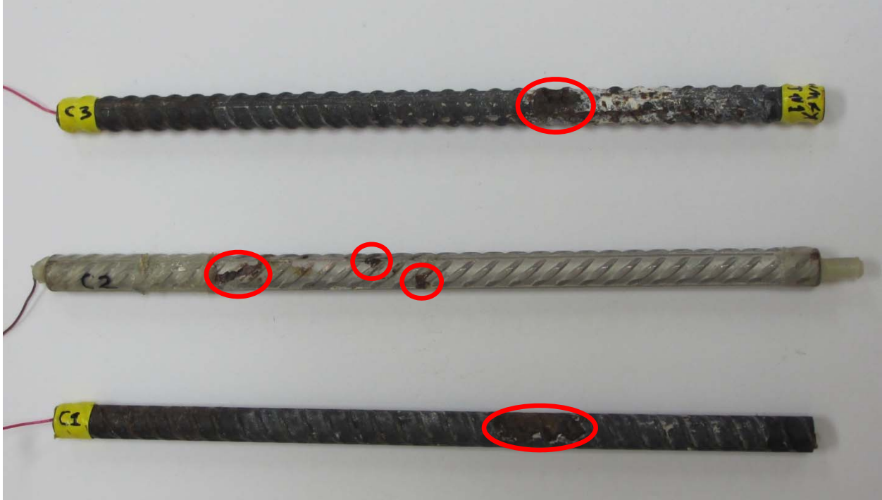
Figure 6.13. Locally corroded rebars (C1, C2, and C3). Red circles show corroded sections.
