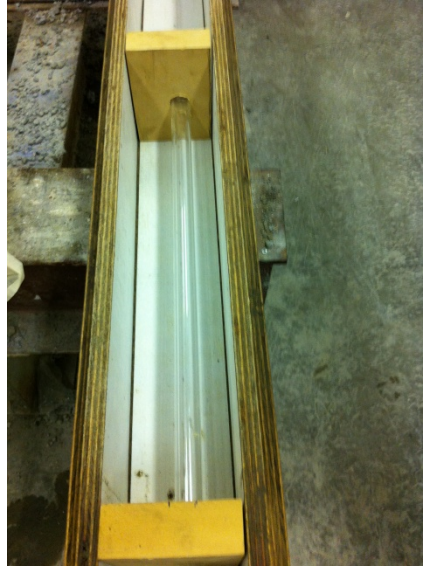
Figure 6.1. Acrylic tube inside the casting mold.
