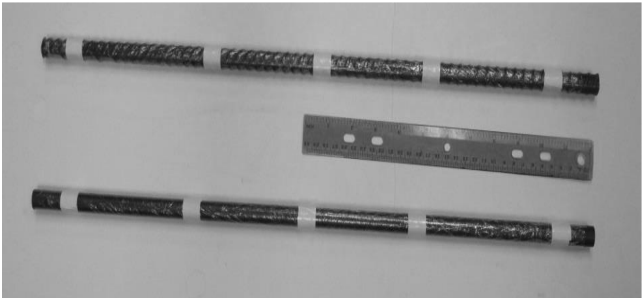
Figure 5.3. Wrapped bar (bottom) and rebar (top) with plastic wrap.
