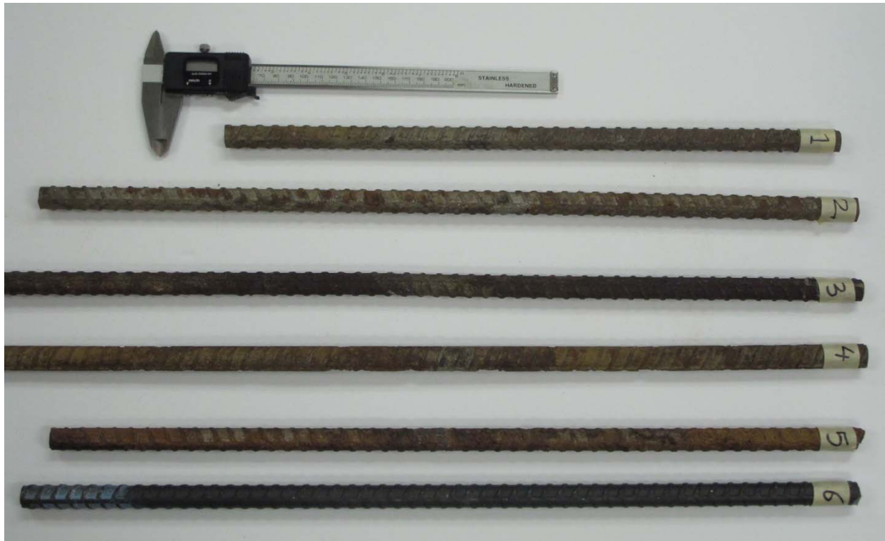
Figure 6.4. Seven bars with different percentages of metal loss.
