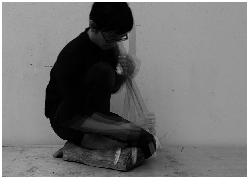
Long Tool Motion Pushing stroke with workpiece secured by body weight Fig. 2.62
