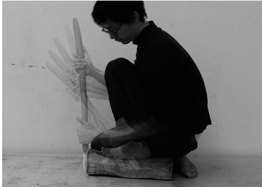
Long Tool Motion Pulling stroke with workpiece secured by body weight Fig. 2.61
