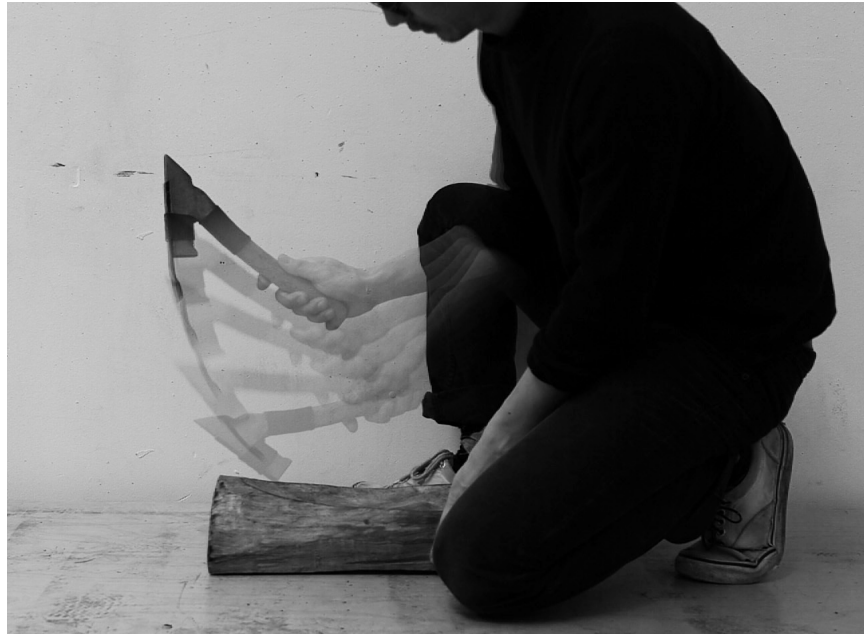
Elbow Adze Motion Fig. 2.49
