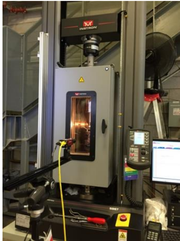
Figure 2.1 The test set-up for the tensile experiments at CanmetMATERIALS (Verma, 2016).
