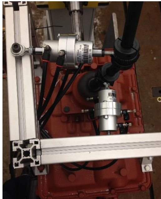
Figure 4-3 Pneumatic system for gear shifting
