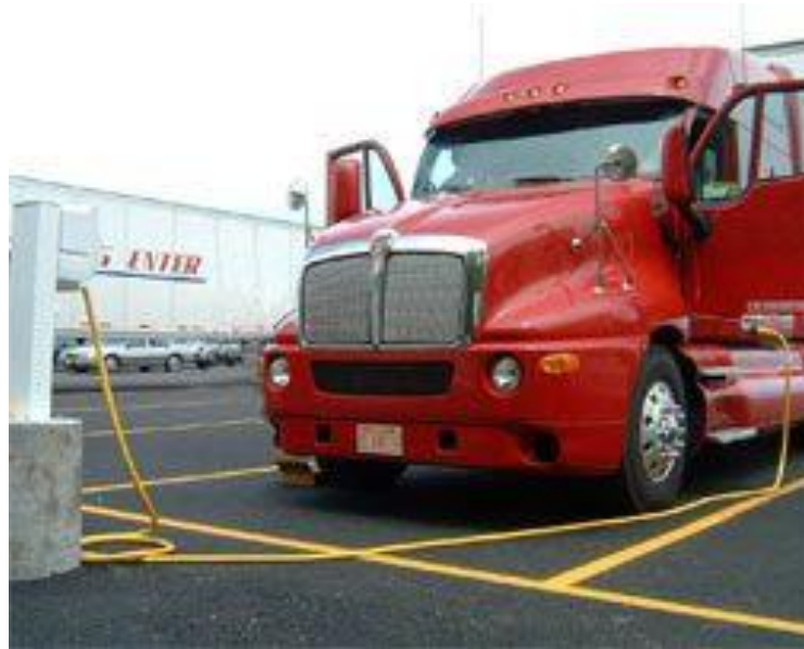
Figure 2-1 Truck stop electrification (TSE), On-board System [8]
