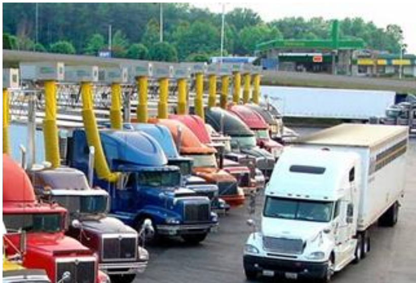
Figure 2-2 Truck stop electrification (TSE), Off-board System [8]
