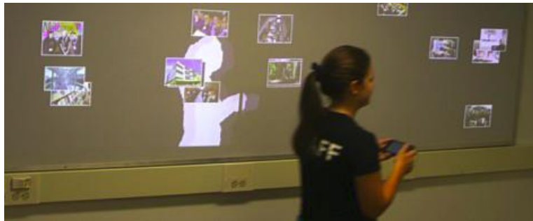
Figure 6-7. User shadow appearing beside the walking person like a mirror. In some cases, slight tracking or display update delays caused the shadow to lag behind the person, placing the shadow outside their peripheral view.
