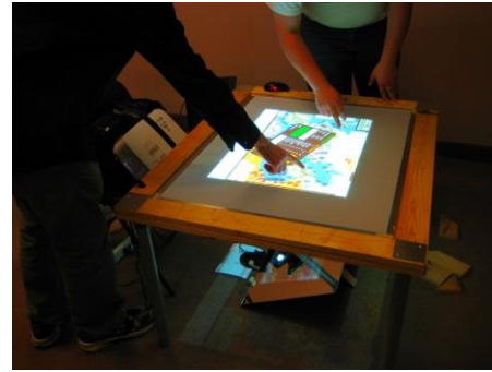
(b) The multi-touch coffee-tabletop surface in action. The IR camera was located at the bottom of the tabletop near the base of the mirror. Lights had to be dimmed to reduce ambient light, and for the projected screen to show.
