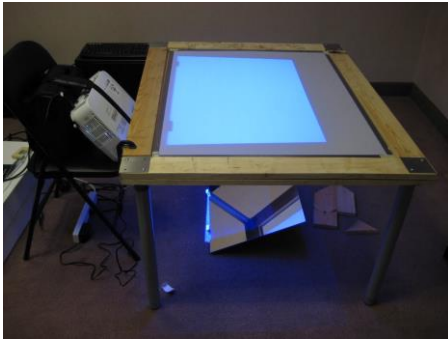
(a) A do-it-yourself multi-touch tabletop interactive surface (built to emulate a coffee table). Because of the lower height the projector had to be fitted at one side of the table, leaving only three free sides for interaction and without any legroom.
