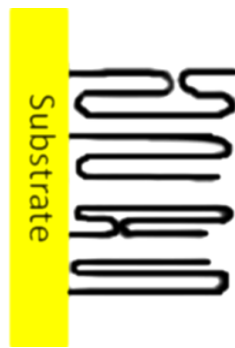
Figure 2.12: Schematic of homeotropic LC configuration of polymer chains. In a homeotropic LC phase, a dense brush forms near the substrate and polymer chains fold back and forth to maintain a high degree of order.
