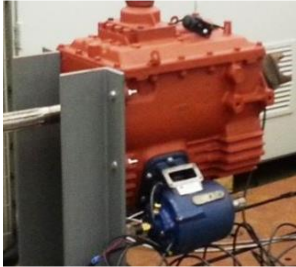
Figure 3-7: “Transmission Aperture” PTO
