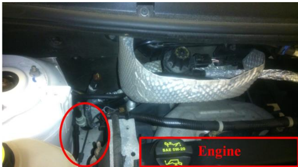
Figure 3-2: Available space to install generator in the low power demand targeted vehicle “Ford Transit Connect Cargo XL-2010”
