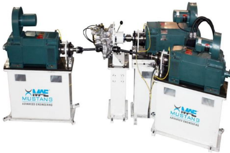
Figure 5-5: Conceptual picture of “Mustang Dynamometer” (HIL test stand) [59]
