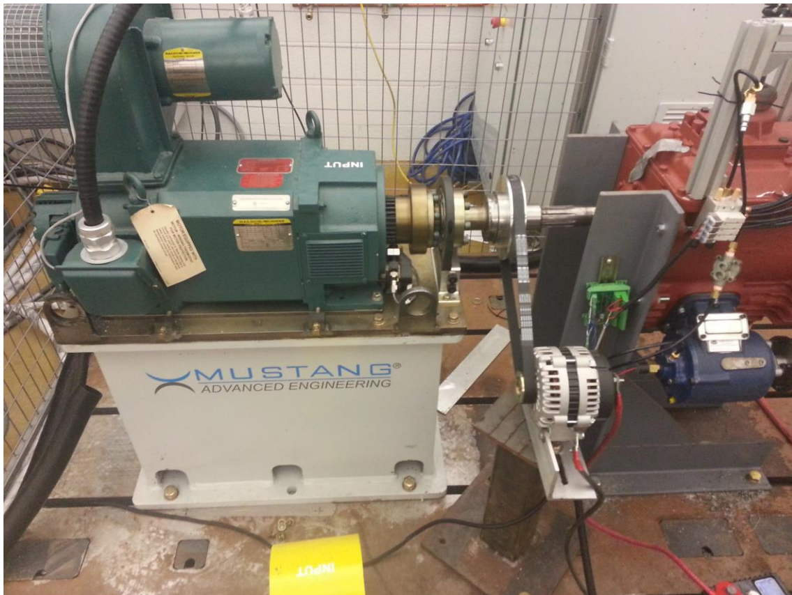
Figure 5-6: Alternator connection to the dynamometer
