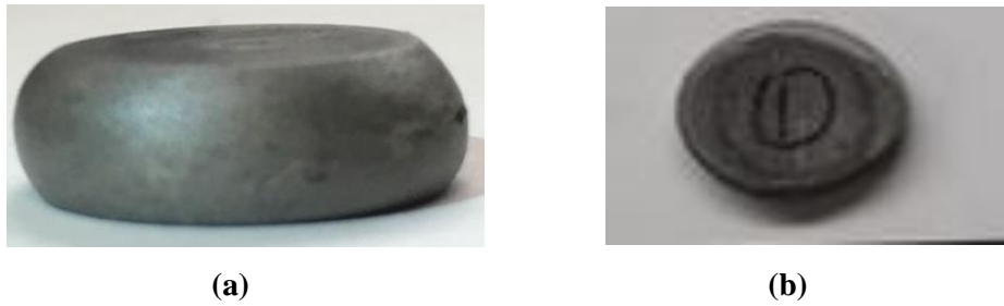
Figure 3.2: Deformation of extruded AZ80 during uniaxial compression @300°C & 0.1 strain/s
