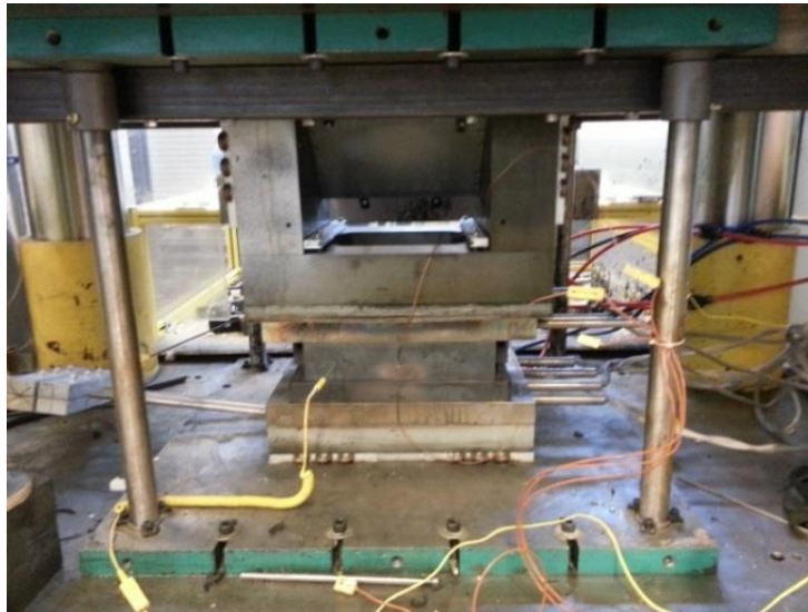
Figure 4.10: 500-ton hydraulic forging press (dies closed)
