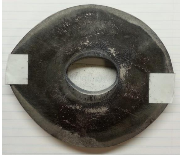
Figure 4.15: Compressed ring using graphite as lubrication with 10mm/min
