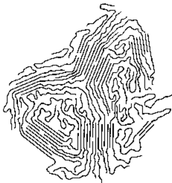
Figure 1.10: Fringed micelle model of semicrystalline polymers, where two domains are shown. Figure from [33].
