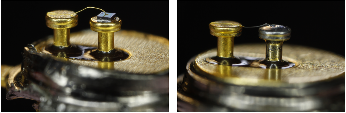
Figure 4.9: Macro photos of the internal structure of the PIN photodiodes. The diode can be seen as the chip on the right post in each picture. The left photo is of an undamaged diode and the one on the right is from external diode test number #2. Photo credit Makarov Lab.
