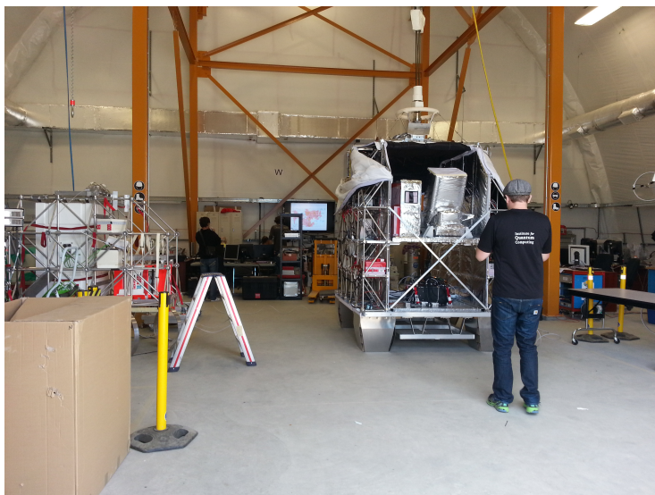
Figure 2.1: Photo taken of the CARMEN gondola used in the 2014 and 2015 Stratos stratospheric balloon campaigns. It has the ability to rotate and point payloads to a specific target with \sim 5^\circ accuracy.
