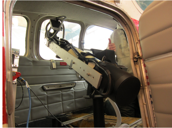
(b) Photo of the installation of the receiver unit in a Beechcraft Bonanza. It can be seen clearly that there is a restricted range of motion within the plane.
