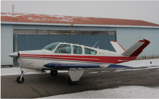
(a) Photo of the Beechcraft Bonanza V-tail that was used for testing and modeling in this chapter. Fun fact: this model is known as the “Doctor-killer” as the tail makes control of the ailerons and the rudder coupled and difficult for beginner pilots. Thanks to Jeff Kehoe for piloting for these tests.
