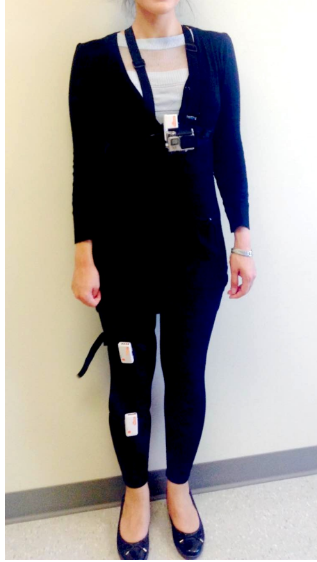
Figure 5.1: The validation process of the system. The subjects wore three SHIMMER sensors along with a GoPro Hero Silver camera and were perturbed in different settings, e.g., on crosswalk, pavement, and tiles.
