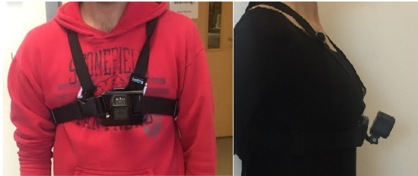
Figure 4.1: The GoPro Hero Session Camera and its chest harness. The camera is facing down to capture terrain features.
