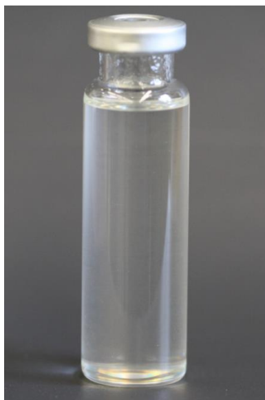
Figure 8-5: Modified CTAB-Triton/c-CNC in toluene.
