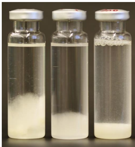
Figure 8-4: Unmodified CNC (left), Triton/c-CNC (center) and CTAB/c-CNC (right) in toluene.
