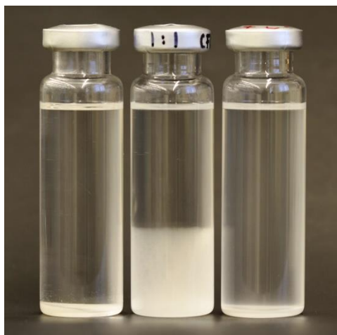
Figure 8-9: Comparison between unmodified CNC (left), CTAB-Triton/Na-CNC 1:1 (center) and the mixture of unmodified Na-CNC with CTAB and Triton (right) in toluene.
