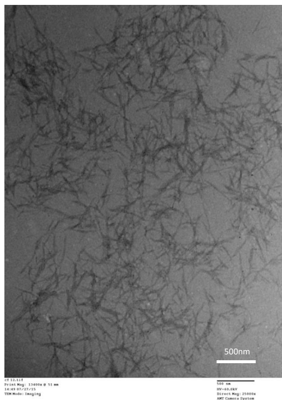
Figure 8-14: TEM image of the unmodified Na-CNC in water.
