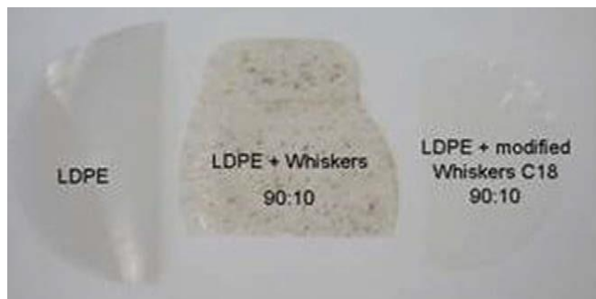
Figure 2-15: Pure LDPE film and films reinforced with 10 wt% of unmodified CNC and CNC modified with stearyl chloride.
