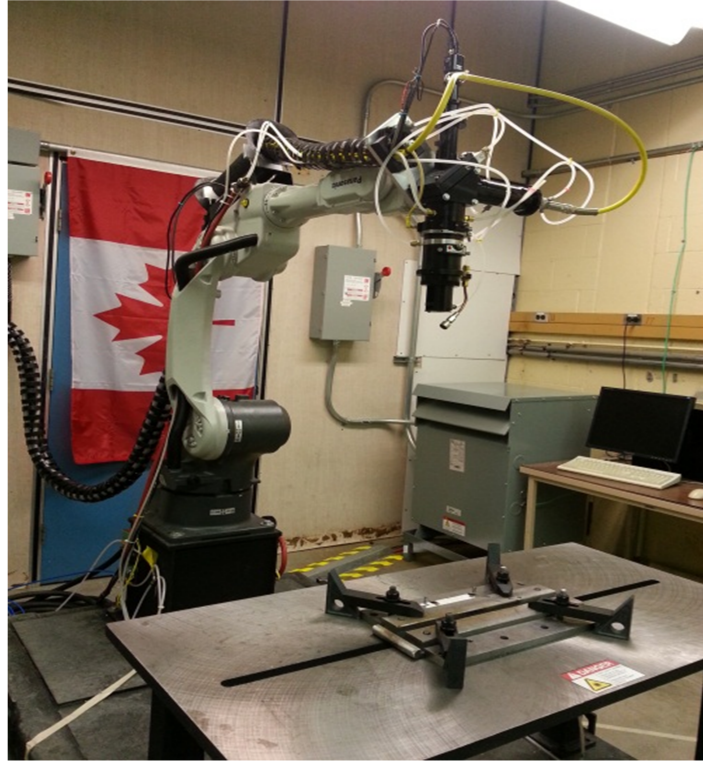
Figure 3.4: IPG Photonics YLS-6000L fiber laser and 6-axis Panasonic robot
