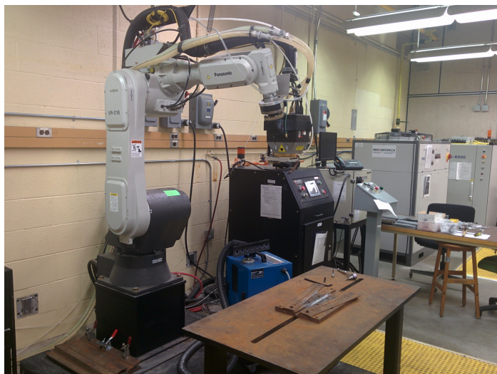
Figure 3.3: Nuvonyx-4000L diode laser and 6-axis Panasonic robot
