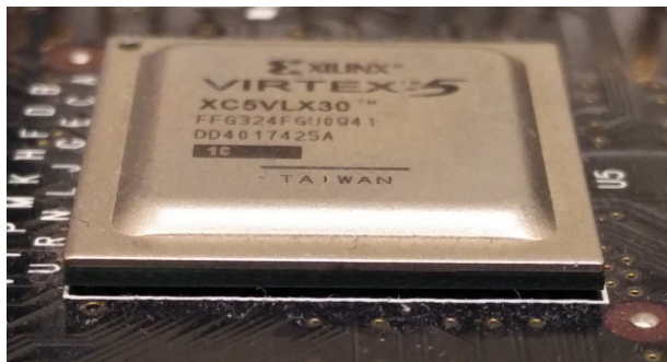
Figure 5.1: A Close Up of the Virtex-5 Cryptographic FPGA showing the Metal Shielding
