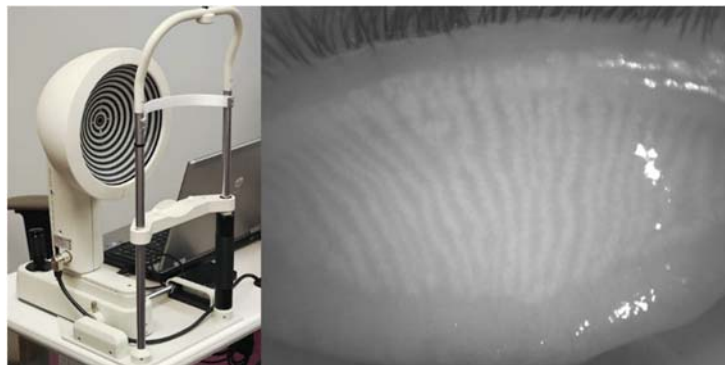
Figure 1-9: The OCULUS Keratograph 4 functions primarily as a corneal topographer, however the infrared diode intended for pupillometry can be used as an infrared illumination source for meibography (left). An everted superior eyelid reveals long thin MGs running vertically on the palpebral side as visualized by the OCULUS Keratograph 4 in infrared light (right).
