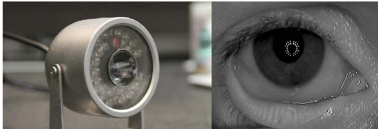
Figure 1-8: Left, an infrared security camera modified for meibography. A ring of infrared LEDs illuminate the eye, and the central camera unit captures infrared video to be displayed on a computer screen (not shown). Right, this image was captured by the modified security camera. The ring configuration of the infrared LEDs of the camera can be seen in the reflection of the cornea. Courtesy of
