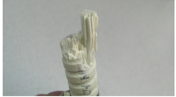
Figure A-29. RB-3: Bottom Bar #12 fracture surface.
