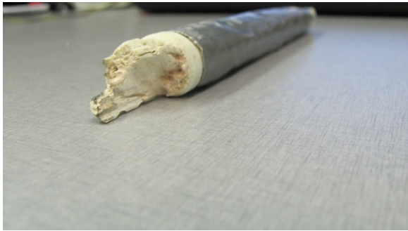
Figure A-9. RB-3: Bottom Bar #1 fracture surface.
