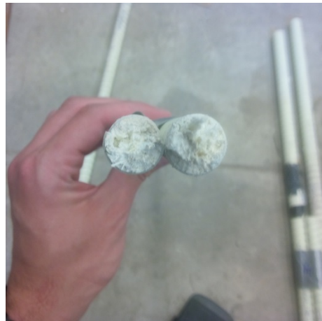
Figure A-41. RB-1: Bottom Bar #1 fracture surface.
