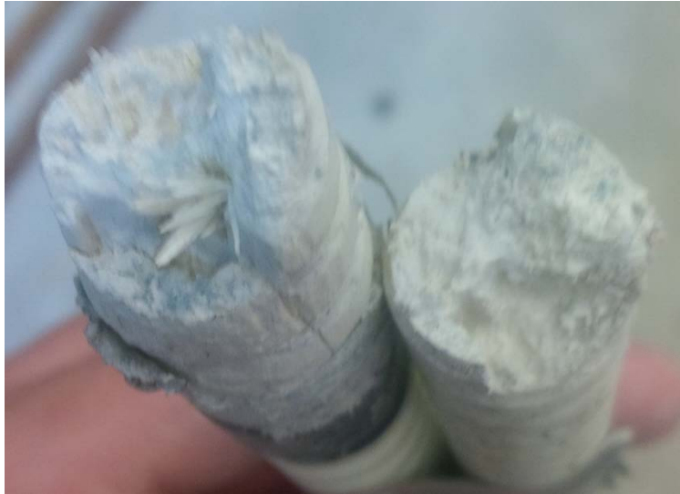
Figure 4-103. RB-1: Failure location of one of the bottom transverse reinforcing bars.
