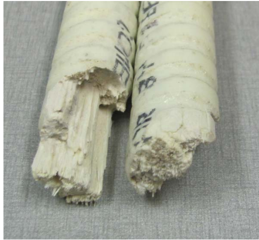
Figure 4-100. RB-3: Broken bar from bottom transverse reinforcement.
