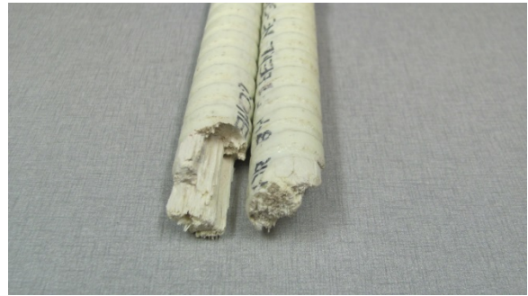
Figure A-11. RB-3: Bottom Bar #2 fracture surface.
