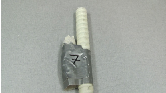
Figure A-20. RB-3: Bottom Bar #7 fracture plane.
