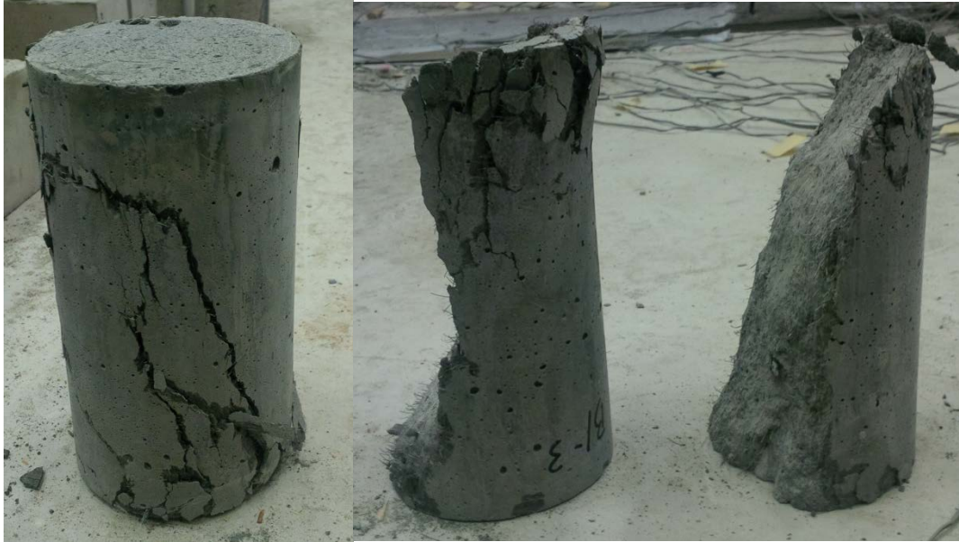
Figure 4-2. Broken UHPC cylinders following compressive cylinder tests. (Left: After failure, Right: After failure and sledge hammer)
