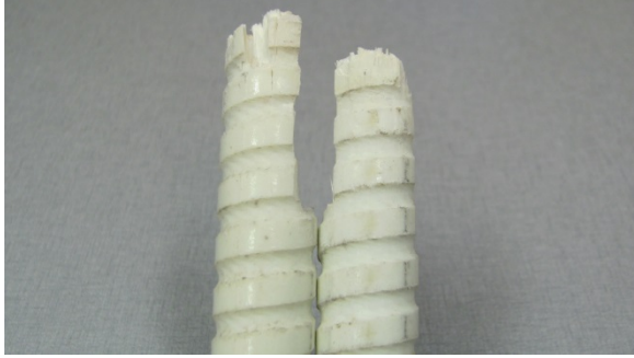
Figure A-12. RB-3: Bottom Bar #3 fracture plane.
