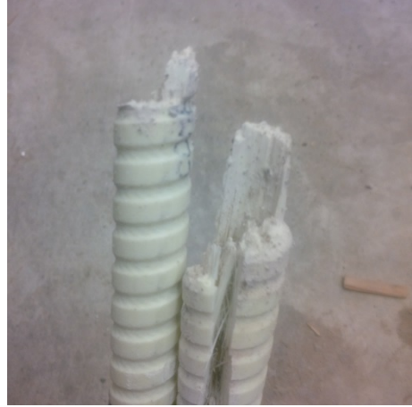
Figure A-58. RB-1: Bottom Bar #10 fracture plane.
