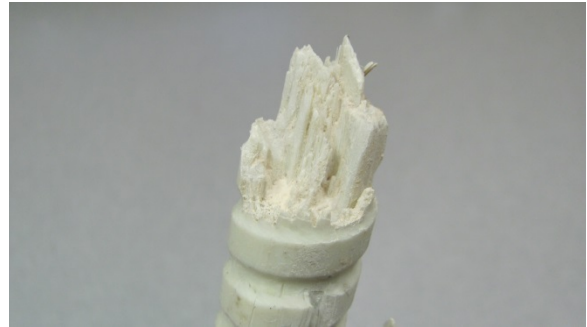
Figure A-25. RB-3: Bottom Bar #10 fracture surface.
