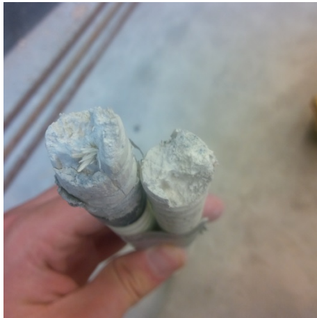
Figure A-51. RB-1: Bottom Bar #6 fracture surface.
