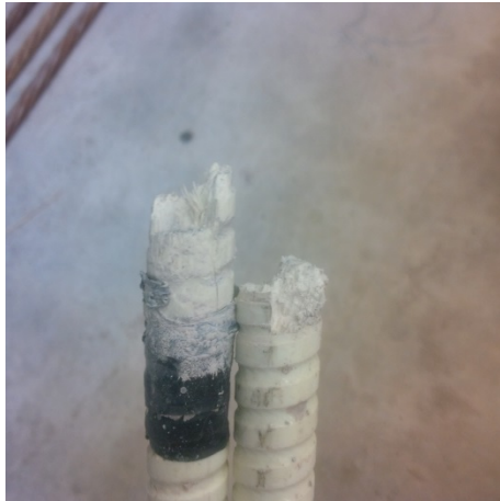
Figure A-50. RB-1: Bottom Bar #6 fracture plane.
