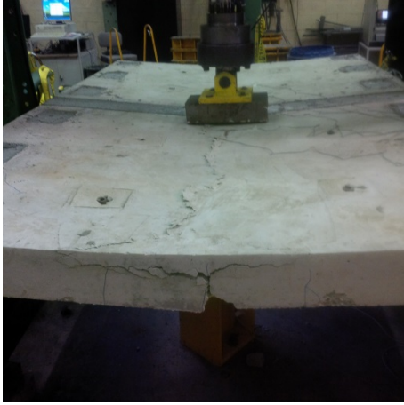
Figure A-37. RB-1: Crushed concrete on top of specimen following failure.
