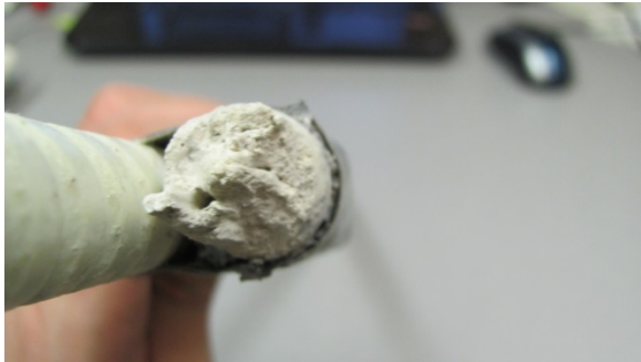
Figure A-21. RB-3: Bottom Bar #8 fracture surface.
