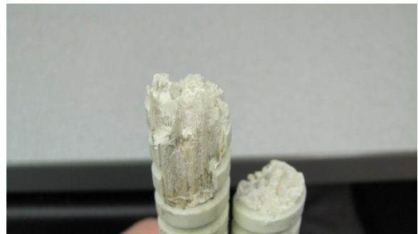
Figure A-19. RB-3: Bottom Bar #6 fracture surface.
