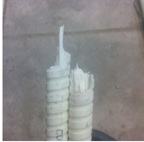
Figure A-40. RB-1: Bottom Bar #1 fracture plane.
