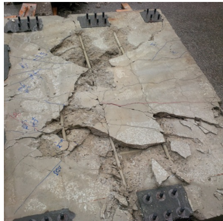
Figure A-6. SB-3: Underside of panel follow punch on centre of panel.
