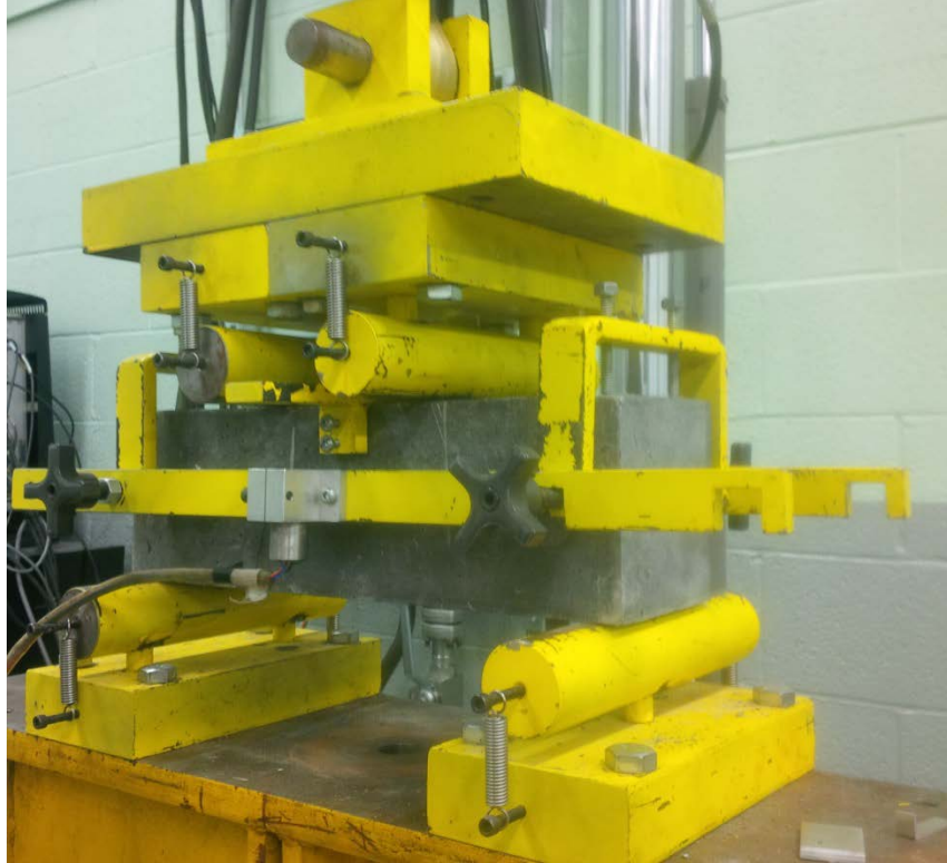
Figure 3-24. ASTM C1609 test setup.
