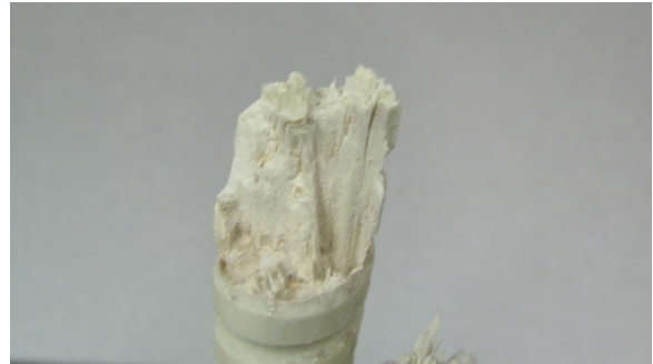
Figure A-17. RB-3: Bottom Bar #5 fracture surface.
