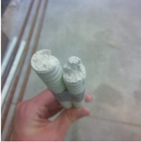
Figure A-43. RB-1: Bottom Bar #2 fracture surface.
