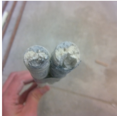
Figure A-53. RB-1: Bottom Bar #7 fracture surface.
