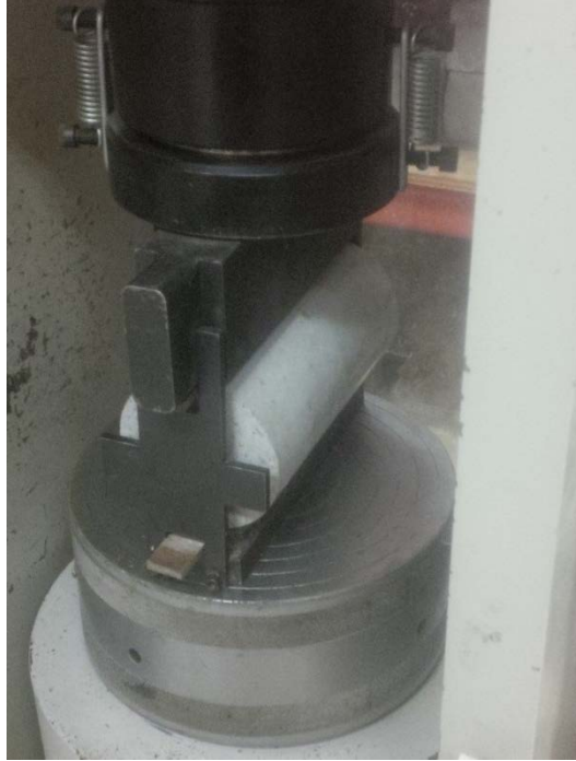
Figure 3-23. Split cylinder test setup.
