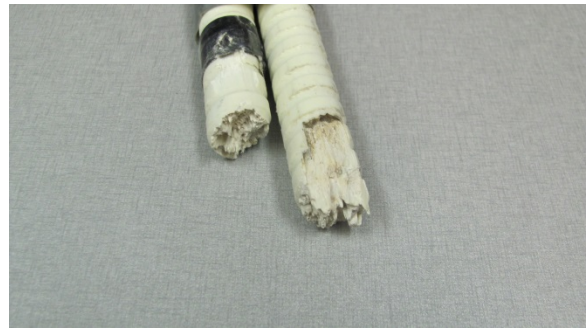
Figure A-18. RB-3: Bottom Bar #6 fracture plane.
