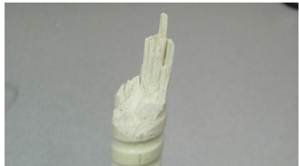
Figure A-27. RB-3: Bottom Bar #11 fracture surface.
