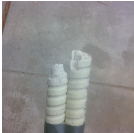
Figure A-42. RB-1: Bottom Bar #2 fracture plane.
