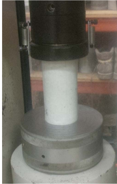
Figure 3-22. Compressive cylinder test setup.
