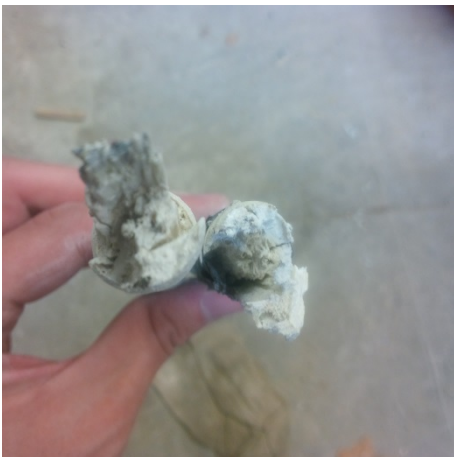
Figure A-57. RB-1: Bottom Bar #9 fracture surface.
