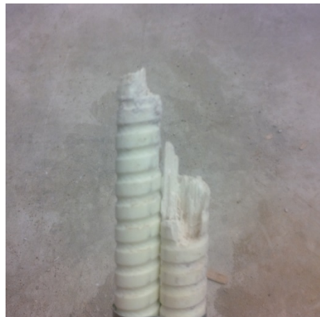
Figure A-60. RB-1: Bottom Bar #11 fracture plane.
