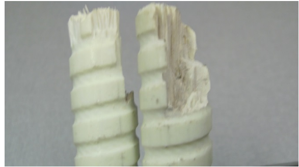
Figure A-10. RB-3: Bottom Bar #2 fracture plane.
