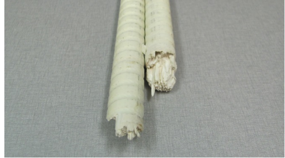
Figure A-24. RB-3: Bottom Bar #10 fracture plane.
