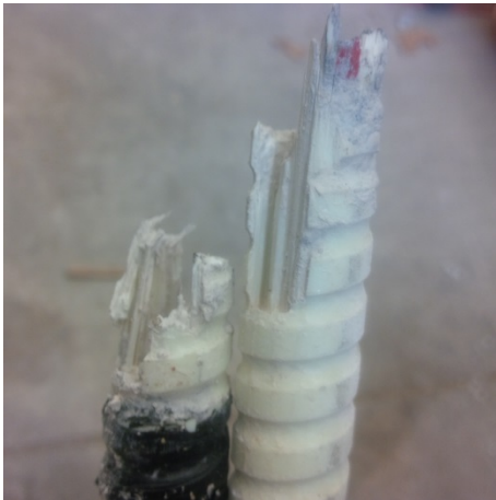
Figure A-56. RB-1: Bottom Bar #9 fracture plane.
