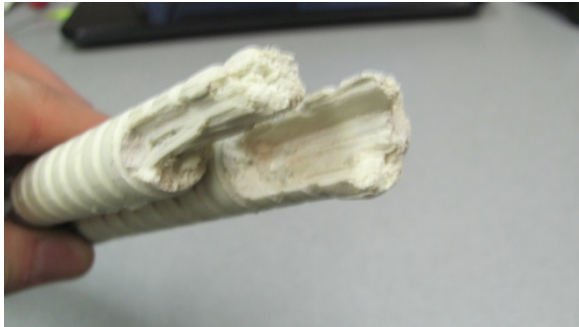
Figure A-13. RB-3: Bottom Bar #3 fracture surface.
