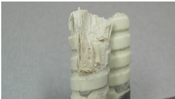
Figure A-23. RB-3: Bottom Bar #9 fracture surface.
