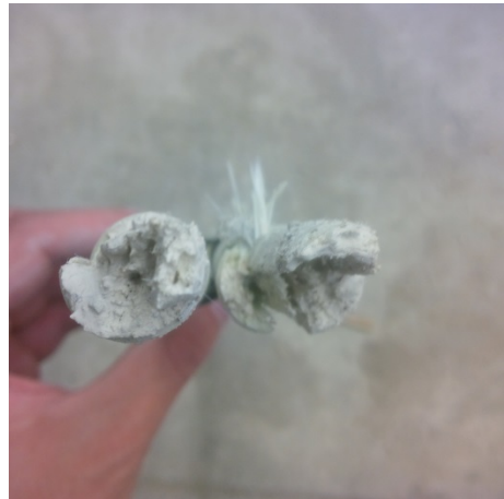
Figure A-59. RB-1: Bottom Bar #10 fracture surface.
