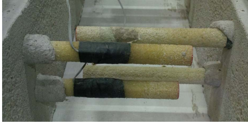
Figure 3-6. Close-up view of sand-coated bars overlapped within the closure strip.
