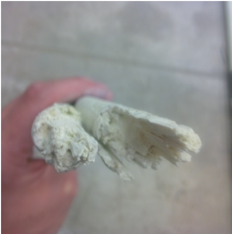
Figure A-45. RB-1: Bottom Bar #3 fracture surface.
