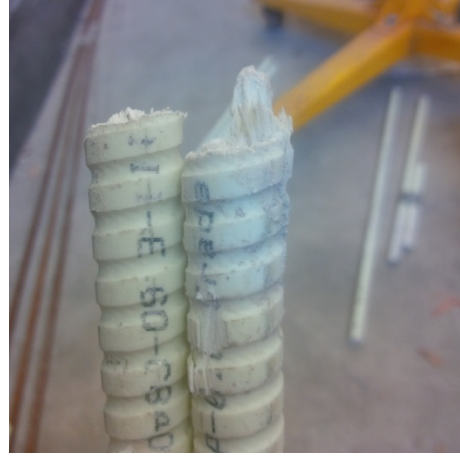
Figure A-46. RB-1: Bottom Bar #4 fracture plane.
