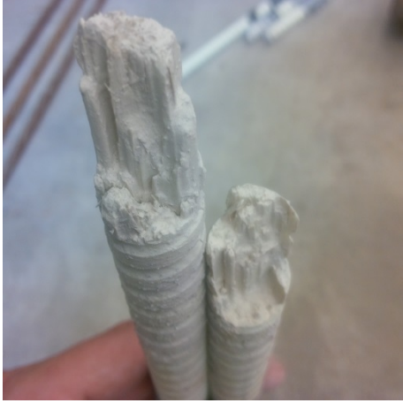
Figure A-49. RB-1: Bottom Bar #5 fracture surface.
