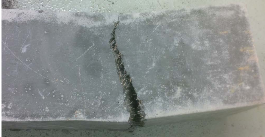
Figure 4-4. Cracked specimen following C1609 prism test.
