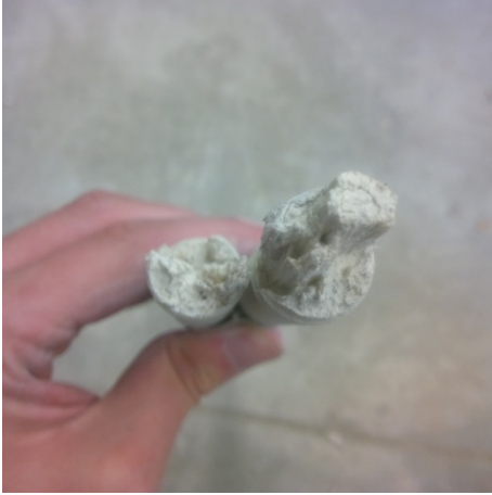
Figure A-61. RB-1: Bottom Bar #11 fracture surface.
