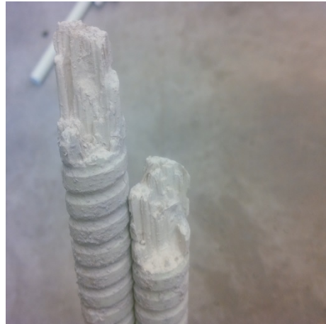
Figure A-48. RB-1: Bottom Bar #5 fracture plane.
