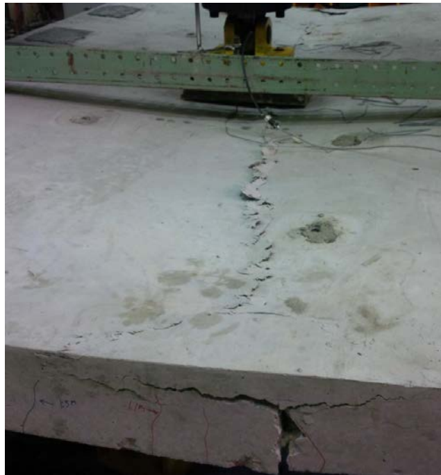
Figure 4-70. RB-3: Concrete crushing failure on top of slab.
