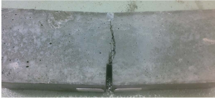
Figure 4-8. Failed notched prism test following loading.
