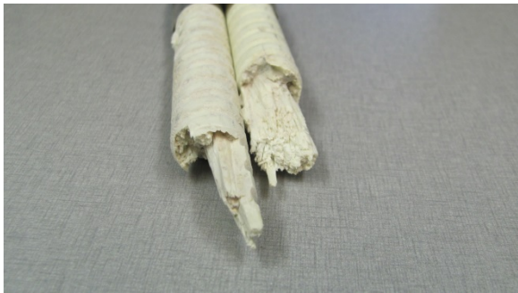
Figure A-14. RB-3: Bottom Bar #4 fracture plane.
