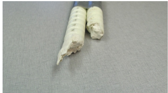
Figure A-26. RB-3: Bottom Bar #11 fracture plane.
