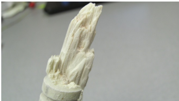
Figure A-15. RB-3: Bottom Bar #4 fracture surface.
