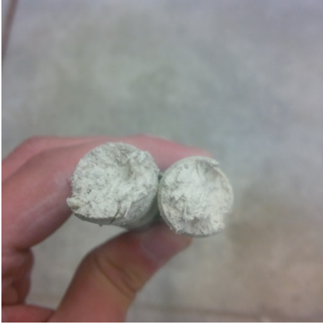
Figure A-55. RB-1: Bottom Bar #8 fracture surface.
