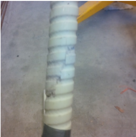
Figure A-62. RB-1: Bottom Bar #12 fracture plane, bar still partially connected.
