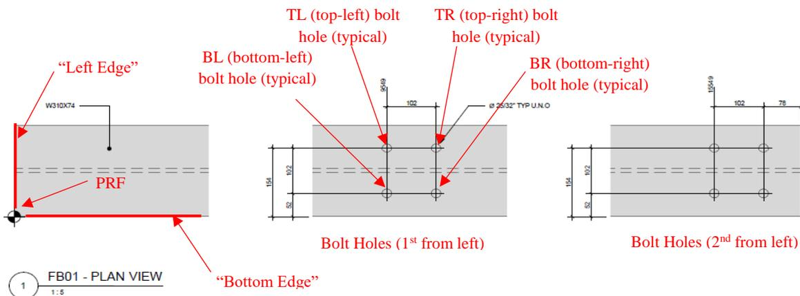
Figure D25: Relevant Information from Shop Drawings for Creating Part Diagram for Floor Beam 1
