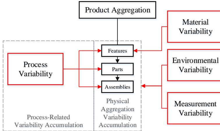
**Figure A4: Primary sources of product aggregation variability accumulation**
