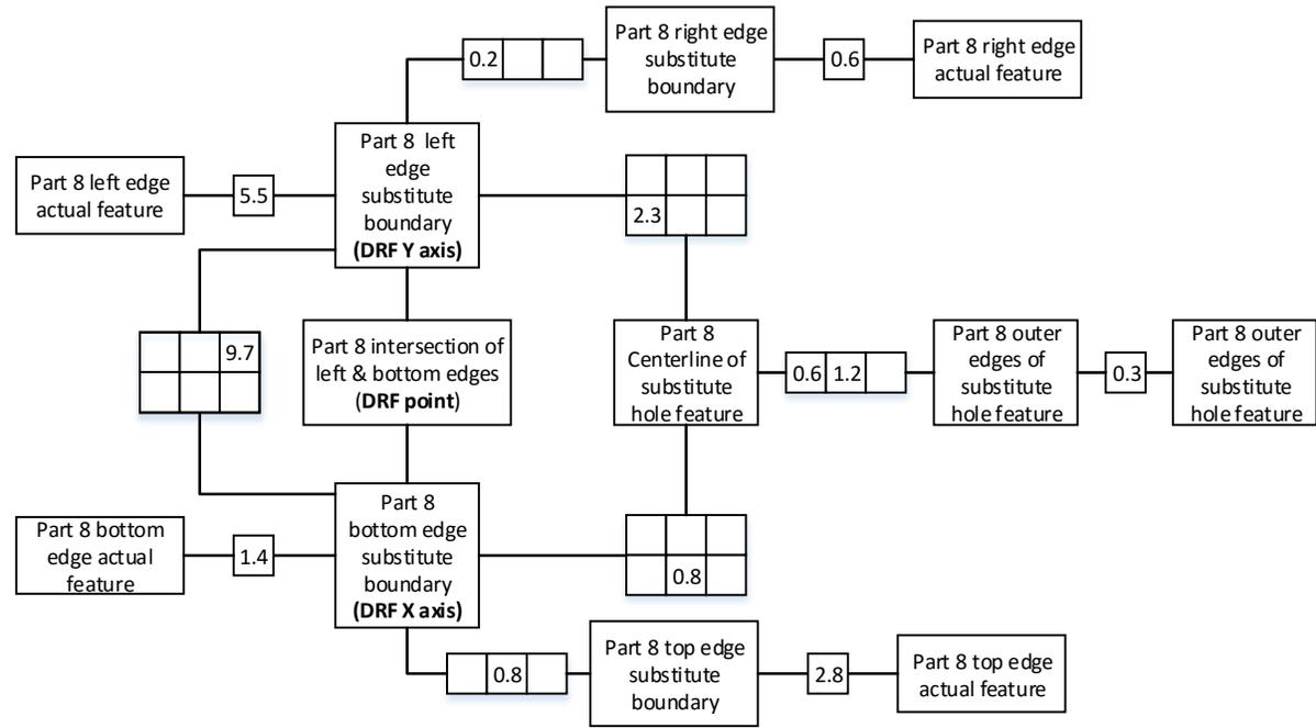
Figure D17: Tolerance Map (above) and Deviation Map (below) for Part 8
