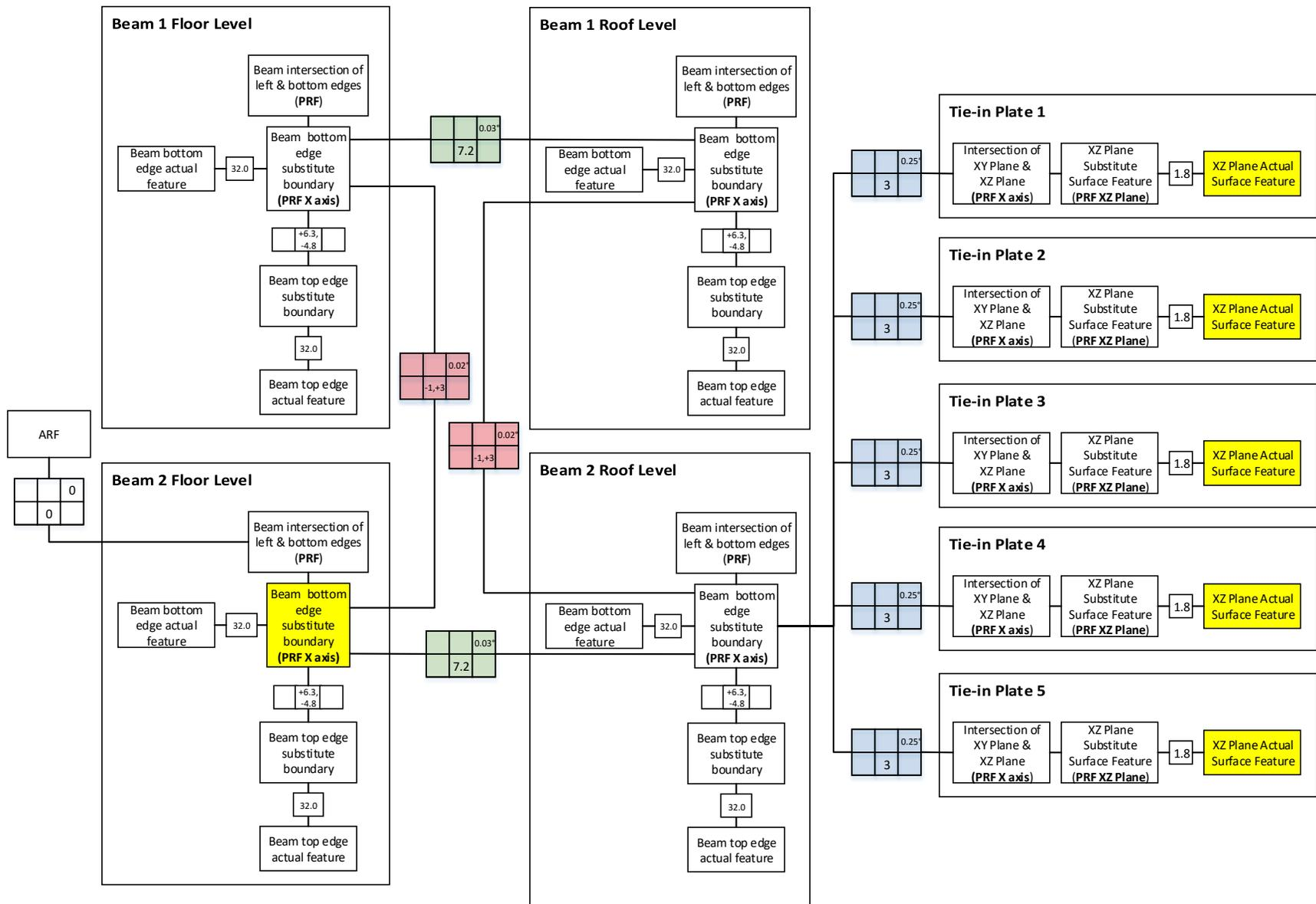
Figure D34: Tolerance Map 1 for Case Study 2 (Tie-in Plate Deviation Analysis)
