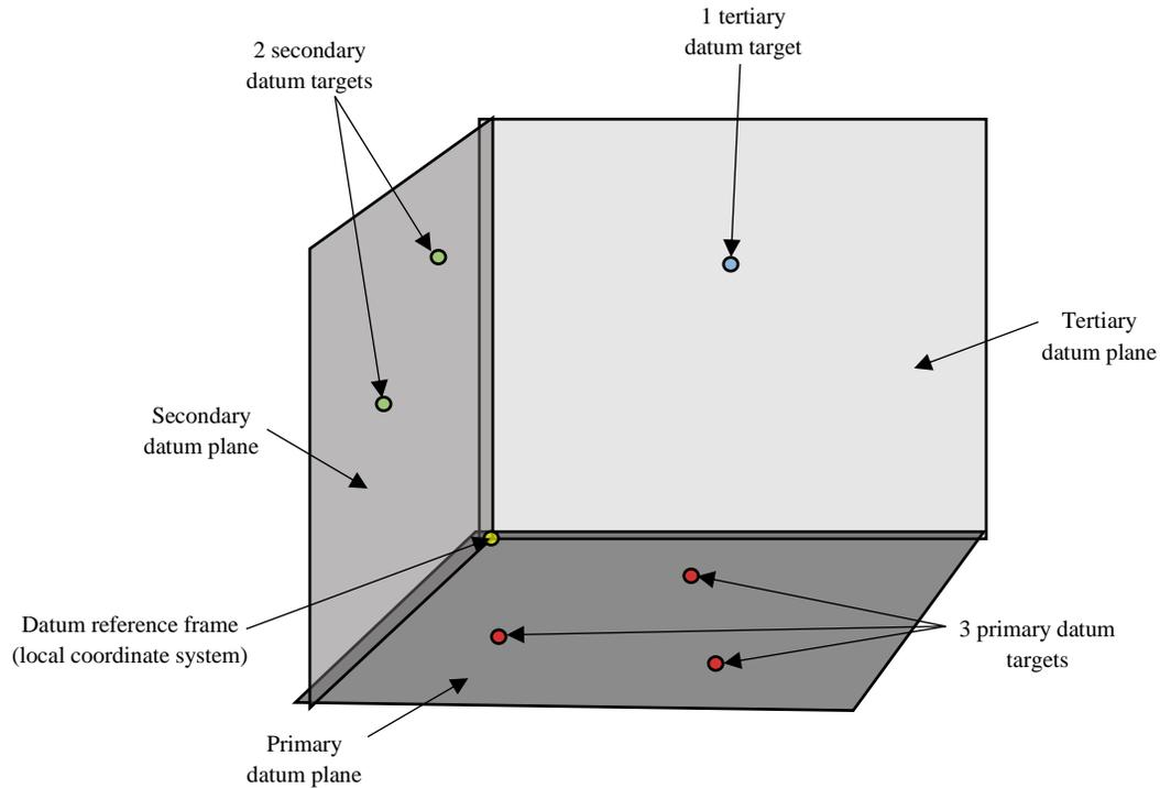
**Figure A9: Depiction of primary, secondary and tertiary datum planes and required targets, adapted from (Hong-Chao Zhang 1997)**
