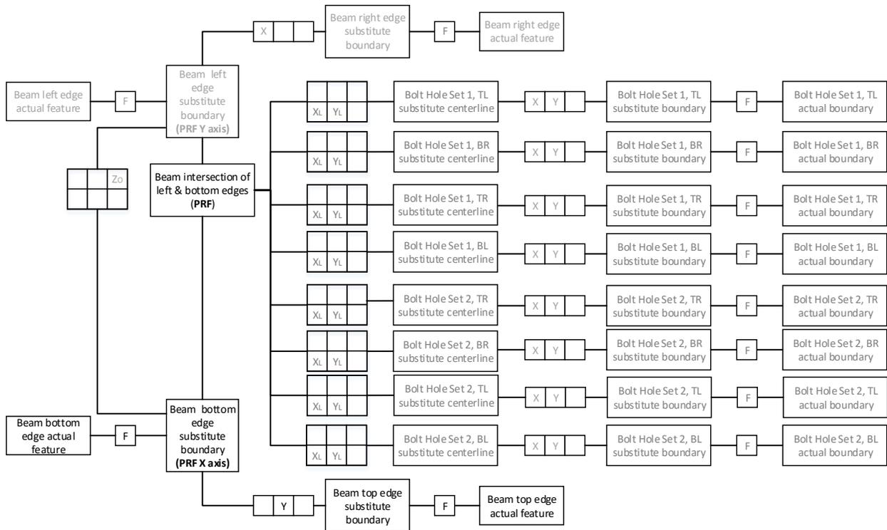
**Figure D26: Part Diagram for Floor Beam 1**
