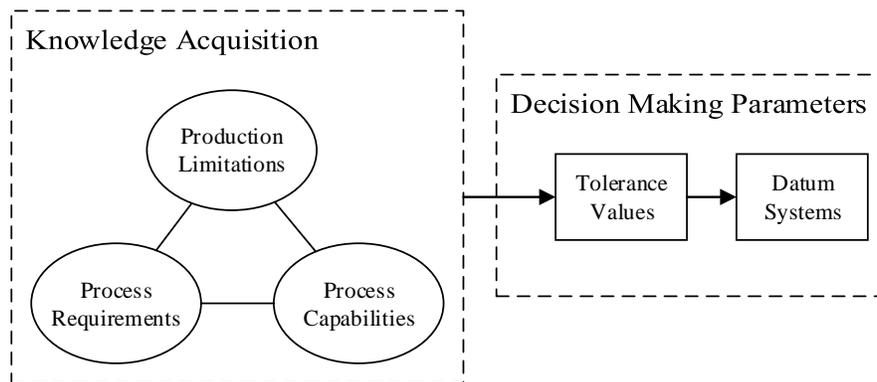
**Figure A6: Sequential information flow for making tolerance-related decisions in manufacturing**
