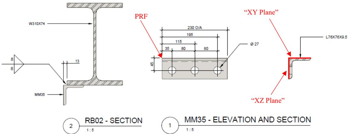
**Figure D29: Relevant Information from Shop Drawings for Creation of Part Diagram for Tie-In Plates**
