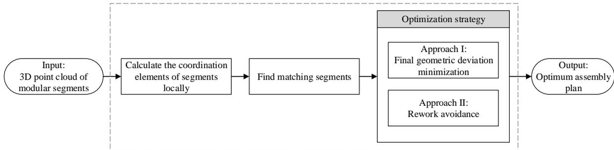
**Figure 82: Framework for optimum assembly planning**
