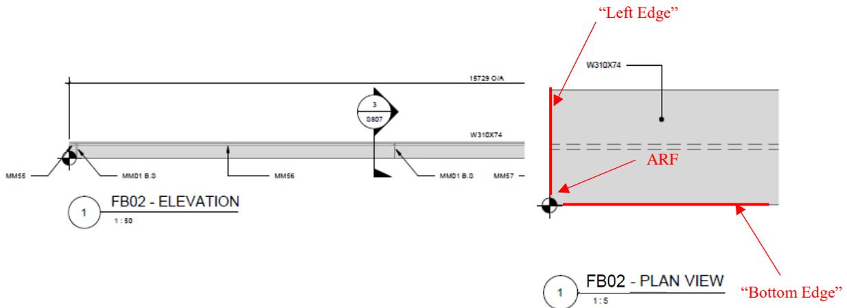
**Figure D27: Relevant Information from Shop Drawings for Creating Part Diagram for Floor Beam 2**
