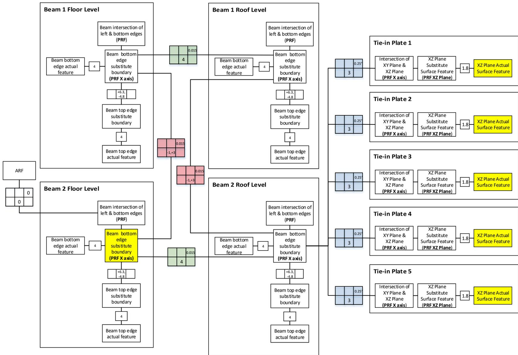
Figure D35: Tolerance Map 2 for Case Study 2 (Tie-in Plate Deviation Analysis)
