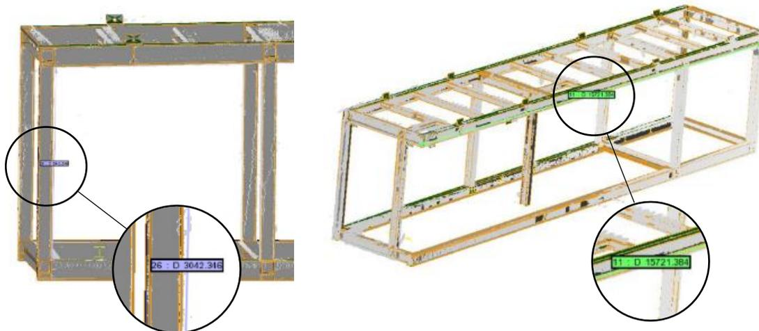
**Figure 74: Sample extracted dimensions (in mm) from 3D point cloud model using PolyWorks®**
