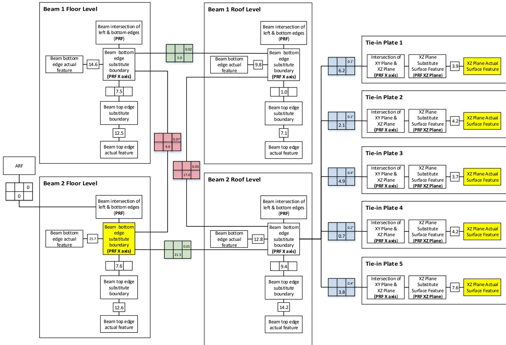
Figure D36: Deviation Map for Case Study 2 (Tie-in Plate Deviation Analysis)
