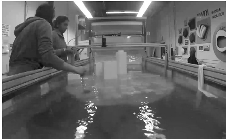
FIGURE 4.9. Turning and Setting up the model in RWDI's Water Flume
