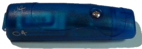
Figure 11: Data logging tri-axial accelerometers mounted to workstations to capture movement of the sit-stand workstation.
